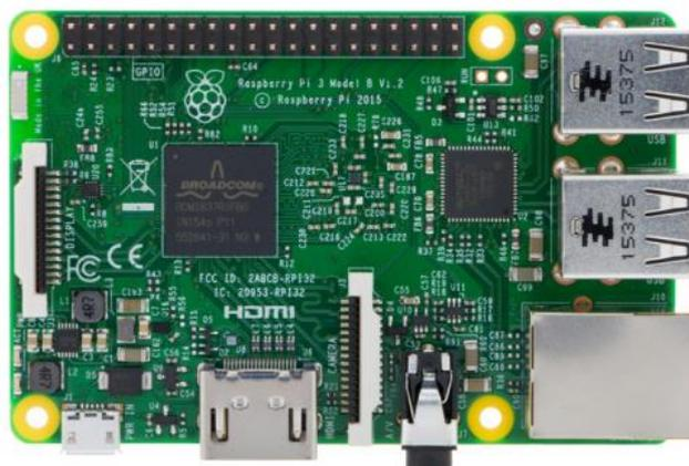
Figura 25: Raspberry Pi 3 Model B v1.2. Fuente [element14.com](http://element14.com)
