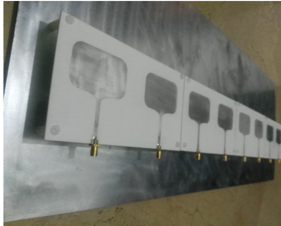
Figure 3.15- 8x1 assembled monopole array
