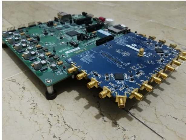
Figure 3.24- FCOMMS5 SDR with ZC702 Xilinx FPGA
