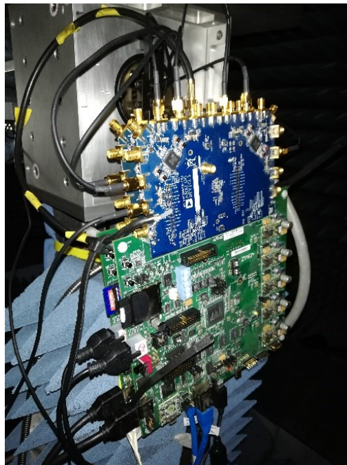
Figure 4.5- 8-elements SDR Unit in Anechoic Chamber
