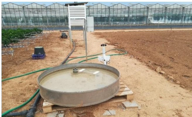
Figure 19. Clase A Pan used in this research to estimate the daily evaporation.
