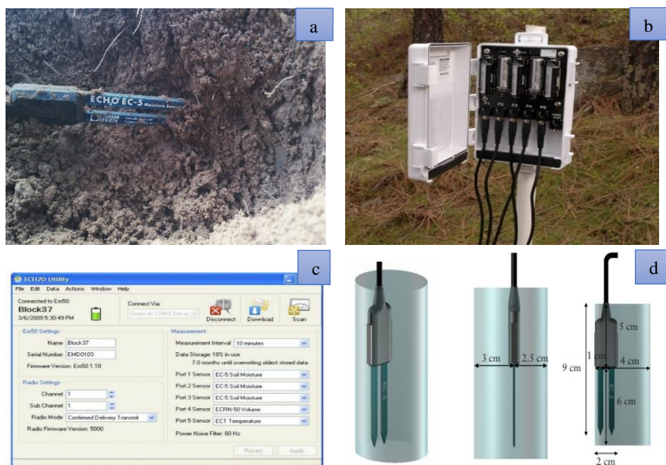
Figure 11. Capacitance probes unit used in these experiments; (a) EC-5 capacitance sensors; (b) Em50 data logger; (c) the ECH 2 O Utility software; (d) EC-5 sensor measurement dimensions.
