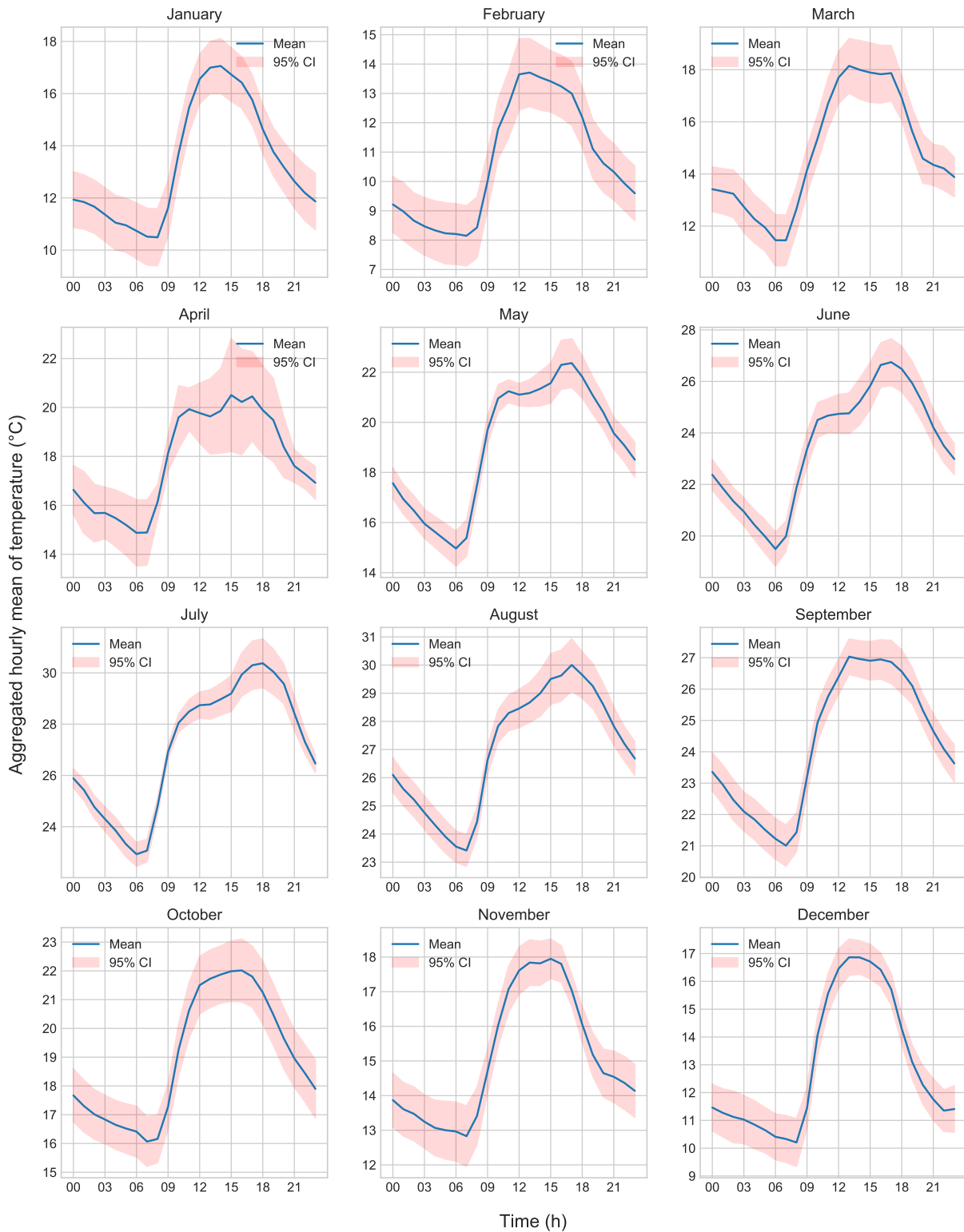
Figure 65: Subplots of the aggregated hourly means of the temperature given in degrees Celsius. Each subplot depicts one month of the year 2018 and contains the hourly mean and its associated 95%-CI band obtained from every of the 24 mean values related to each hour of the day from 0 to 23 hours.
