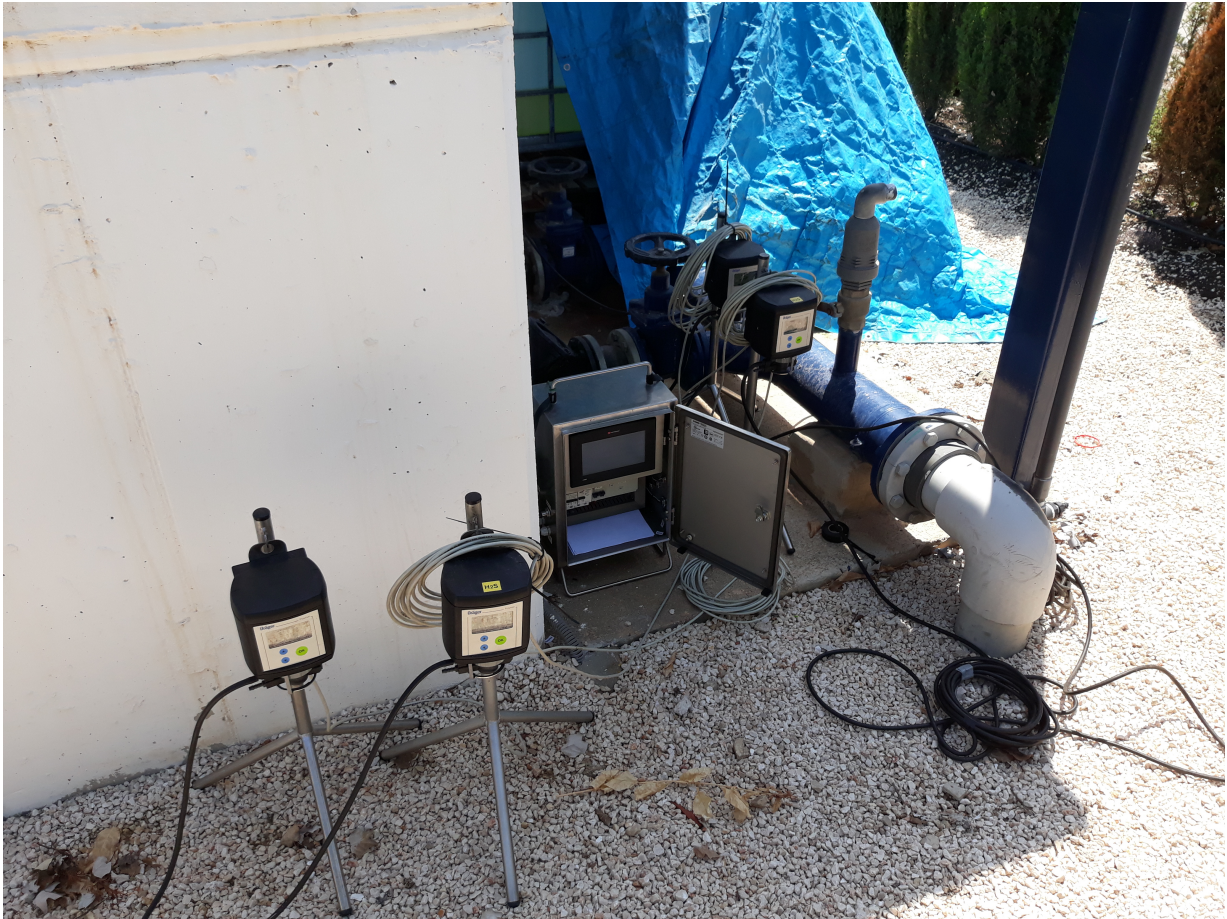
Figure 31: Photograph of the Dräger Polytron 7000 gas measuring devices situated in the shade along with their associated data register. The black cables represent the air-sucking system transporting the odorant-laden air to the sensors, which then send their measurement result digitally via the light gray cables to the registry.
