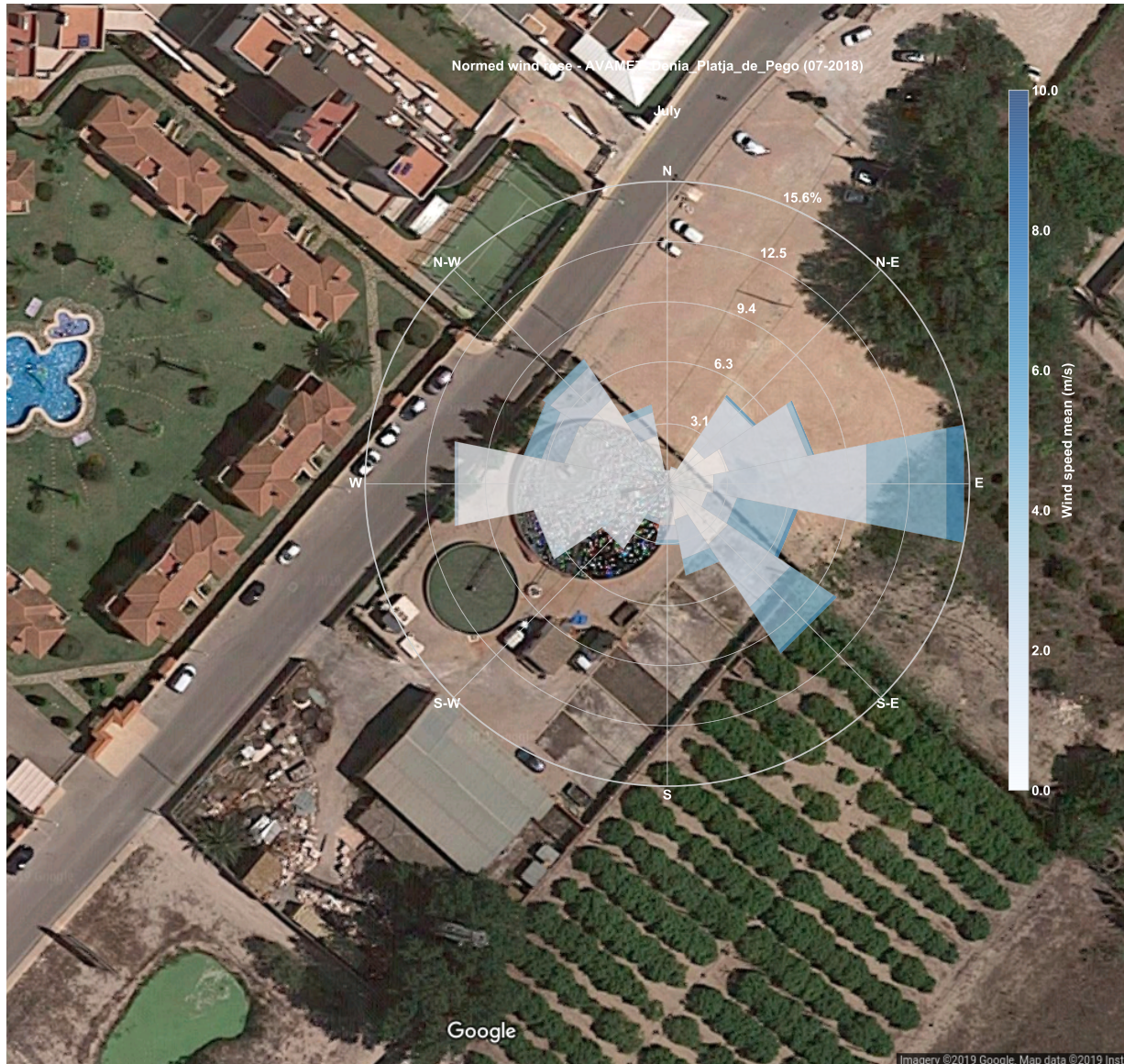
Figure 68: Wind rose displaying the wind speeds occurred in July 2018 from light to dark blue in m/s and the corresponding wind directions divided in the 8 main compass points N, N-E, E, S-E, S, S-W, W and N-W starting from the North "N" clockwise over East "E" and South "S" to West "W". The graph is overlaid on top of the satellite picture from Google Maps showing the top view of the WWTP and its surroundings, including the affected dwellings in between WSW and NNW. Furthermore, the concentric rings are labeled with the percentages each of the plotted bars comprises with respect to the totality of wind speed observations of the dataset.
