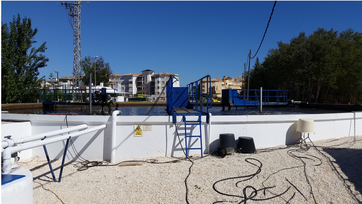
Figure 32: In this photograph, the makeshift sun protection of the sensors by utilizing plastic buckets is demonstrated. To that end, they were slipped over the top of them. Besides, in the left part of the picture one can locate the sensor cables which were fixed by the weight of a medium-sized brick put on top of them. As for the weight, the cables are still passable. To ensure this, the endings of the sensor cables always protruded a few centimeters from the brick.
