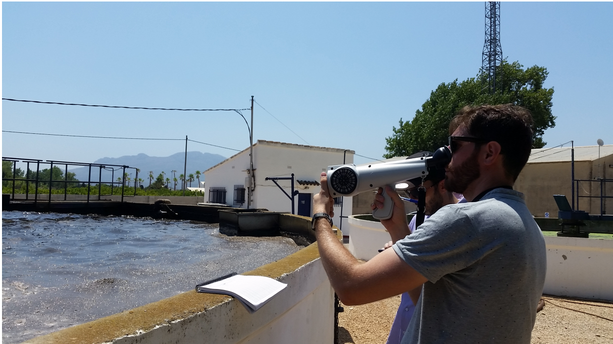
Figure 37: Close-up shot during dynamic field olfactometry measurements on the WWTP site using the Nasal Ranger equipment (see fig. 35) on 3 August 2018. Here, the outgoing odors from the bioreactor toward the closest dwellings were measured.
