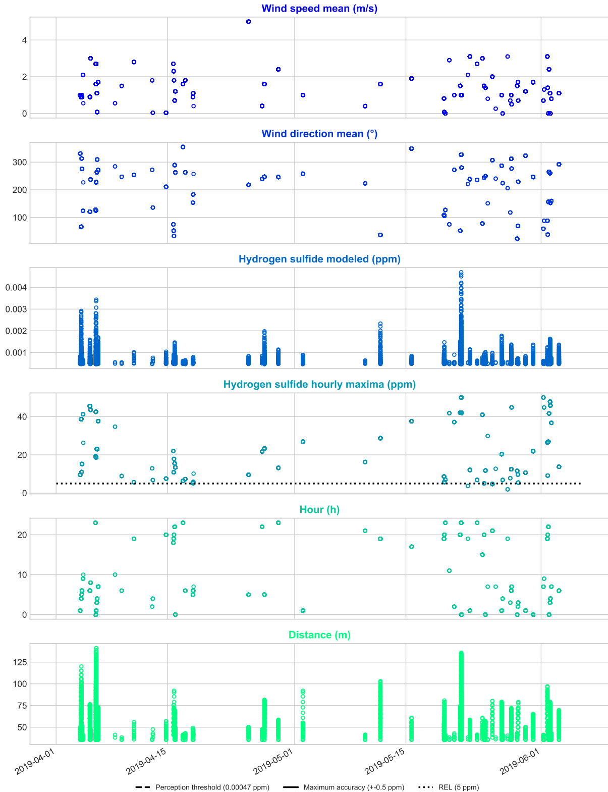
Figure 93: In this figure, each time series belongs to one of the characteristic variables; namely wind speed in m/s and wind direction in angular degrees, modeled hydrogen sulfide concentrations and the corresponding input maxima in ppm, the associated hour and distance in meters to the main emission source of each event. The modeled hydrogen sulfide concentrations stem from the alternative model approach, and is filtered both by the residential area of interest (see map 89) and by the perception threshold of 0.00047 ppm (see 2.2.3). All the other variables belong to these double-filtered model concentrations from the the last measurement period from 3 April to 3 June 2019. With regard to the legend, particular concentration limits in ppm are embedded where suitable; namely the recommended long-term exposure limit (or long-term REL) and perception threshold of the odorant, mentioned in subsection 2.2.3, and the maximum accuracy of the deployed measuring instruments explained in 3.1.1.
