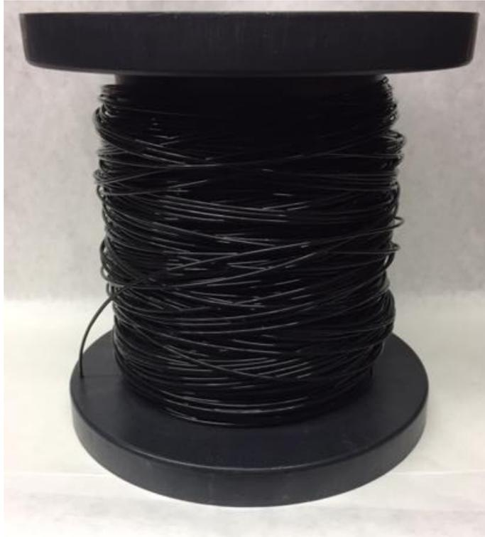
Fig. 63. Monofilamento de PLA + 5% Carbon Black.
