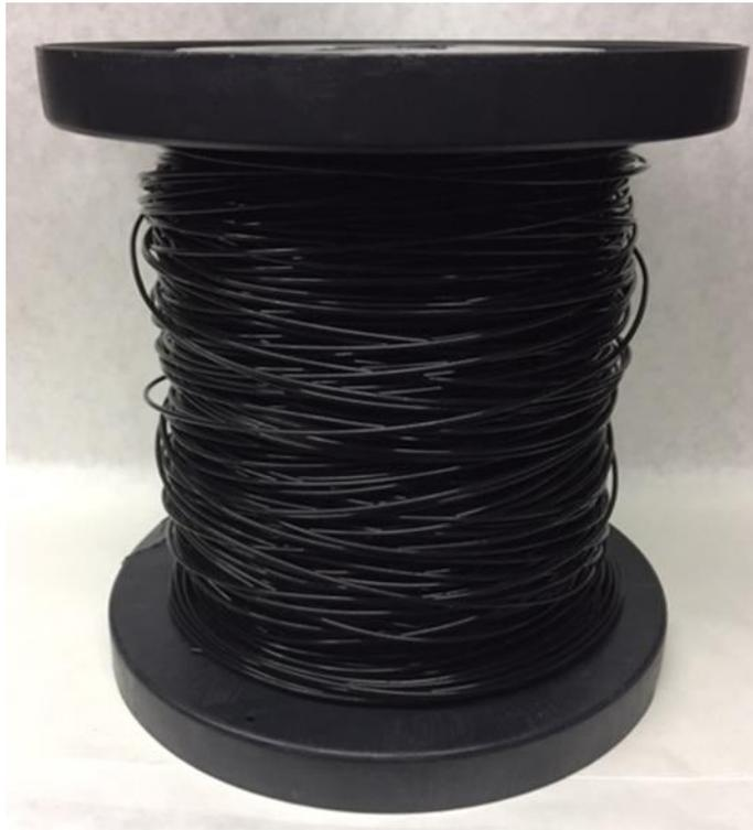
*Fig. 62. Monofilamento de PLA + 10% Carbon Black.*
