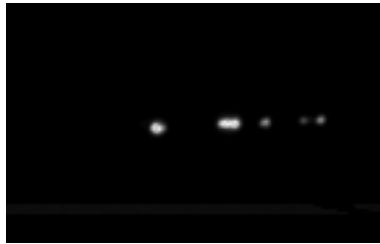
Figure 4.5. Image of recorded plasma obtained during the laser induction system optimization test. This image has been recorded in ambient air condition and shows an example of a multipoint induction event.
