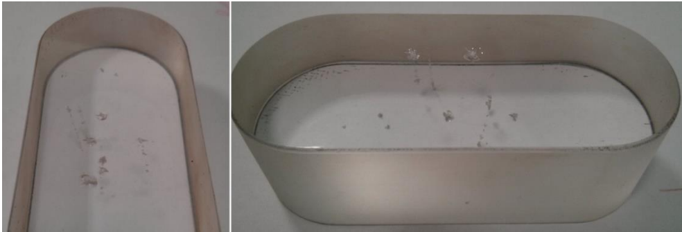
Figure 4.2. Pictures of an optical access windows as damaged by the laser beam focused trough it under engine-like conditions, at 532 nm and with 350 mW of peak power.
