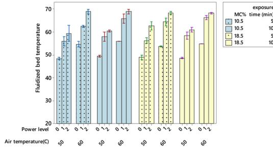
**Figure 5** Final bed temperature at two set air temperatures of 50 and 60°C, two exposure times of 5 and 10 min, microwave powers of 0, 300, 400W for 18.5% MC (power level of 0, 1, 2 respectively) and 0, 400, 500W for 10.5% MC (power level of 0, 1, 2 respectively); bars are SE from the mean; MC-moisture content
