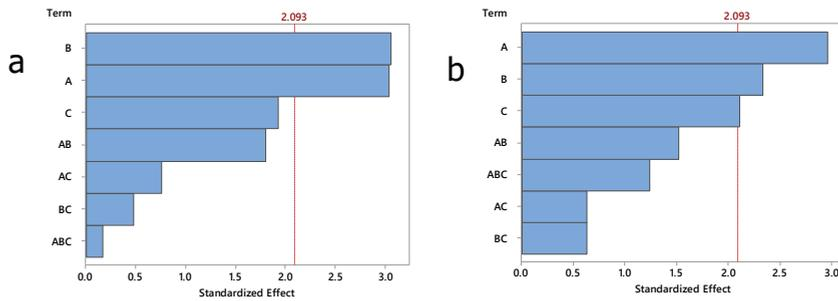
**Figure 6** Pareto Chart of the standardized effects for (a) germination percentage and (b) infected seeds percentage counted after 4d of lentil seeds at 18.5% MC; A = microwave power (0, 300, 400 W), B = air set temperature (50, 60 °C), C = exposure time (5, 10 min);  $\alpha = 0.05$
