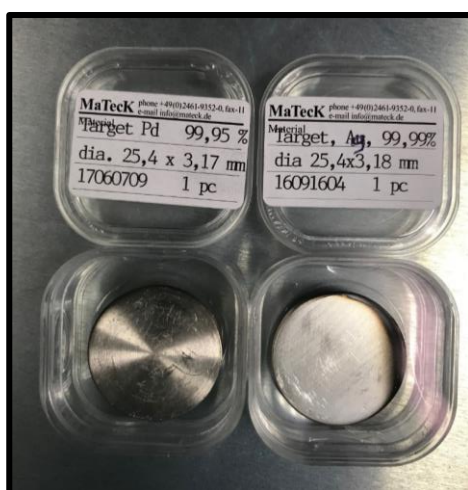
Figure 6: MaTeck metallic palladium and silver targets used for sputtering deposition
