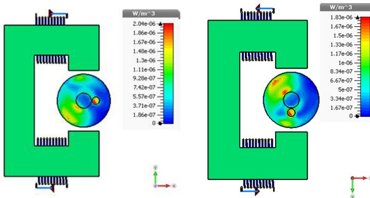
Fig. 6. a) power loss density in tissue in right-position, b) power loss density in tissue in center-position.
