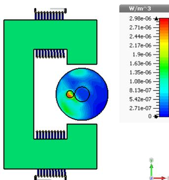
Fig. 5. power loss density in tissue in left-position.
