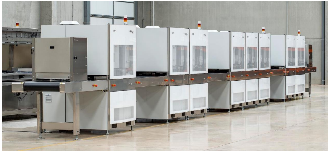
Figure 4: In-line Kerajet ink-jet printers for ceramic tile decoration. [Online] Available: https://www.kerajet.com
