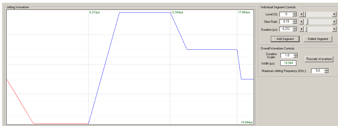
Figure 26: Designed and applied waveform in for the jetting of solvent-based silver ink droplets via ink-jet printing with a Dimatix DMP Series printer.
