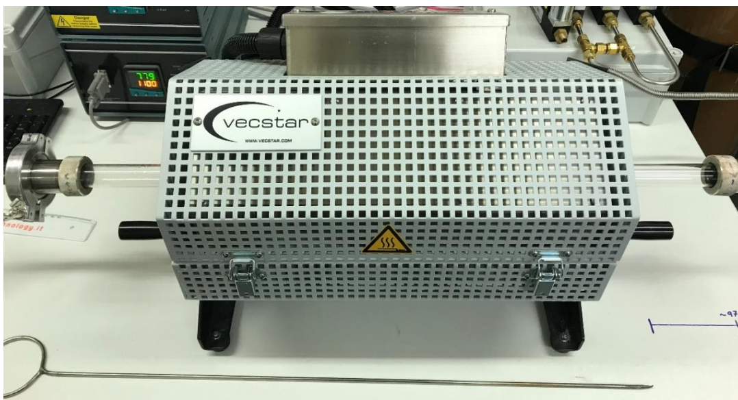
Figure 21: Tube furnace utilised for the sintering of porcelain stoneware substrates.
