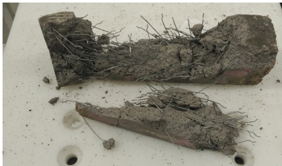
Fig. 6. Appearance of the water saturated HE_1 mortar after 2min under induction heating.
