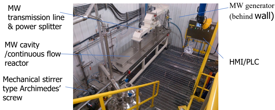
Fig. 2. Continuous-Flow Industrial-Scale MAP™ Extractor in ATEX environment
