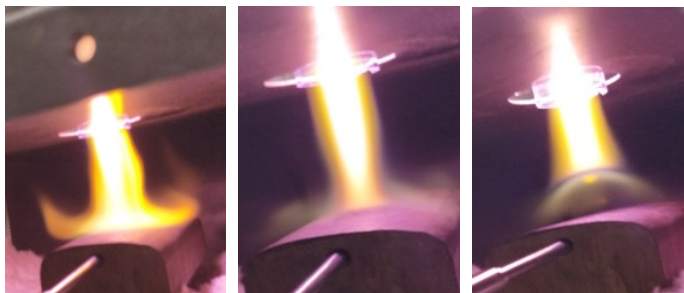
Fig. 4. Effect of gas flow on plasma afterglow delivery at 2kW
