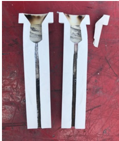
Fig. 5. Thermal shock damage of the AlN tube
