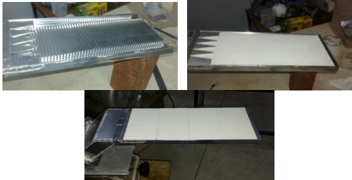
Fig. 1. Comb applicator (left) without covering with ceramic plates. Ceramic applicator (middle) without covering by ceramic plates. Comb and ceramic applicators view (right) covered by ceramic plates (3x84x146 mm - 4pc).
