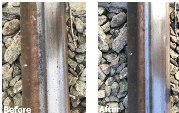
Fig. 13. Effect on railhead oxidation
