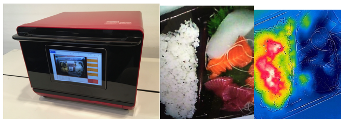
Figure 8. (Top) Photo of intelligent cooker, (bottom left) photo of Sushi (Raw fish) lunch box, (bottom right) The rice warms up to the set temperature and the sushi (raw fish) doesn't warm up at all (thermographic image).
