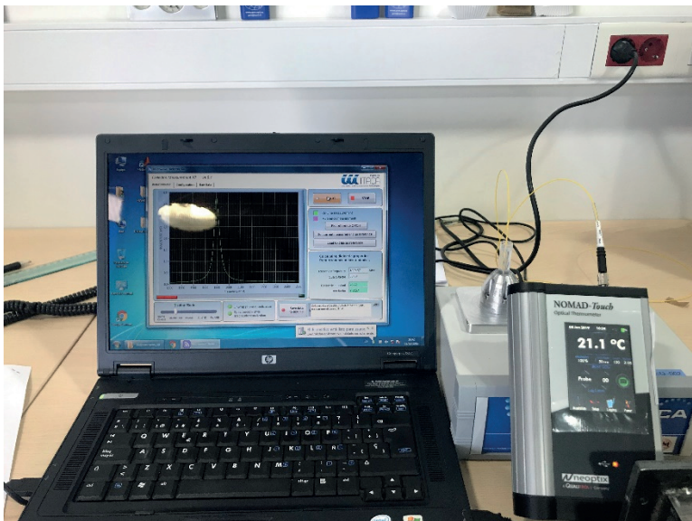
Fig. 1. Set up for the dielectrometer with a fiber optic temperature probe.
