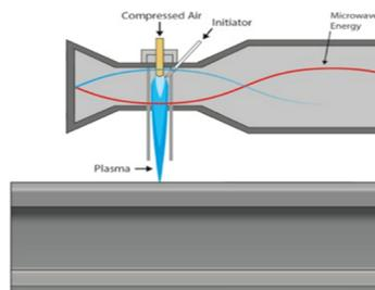
Fig. 2. Plasma Head Cross-section Schematic
