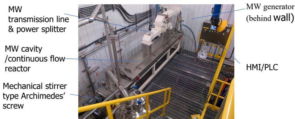
**Fig. 2.** Continuous-Flow Industrial-Scale MAP™ Extractor in ATEX environment
