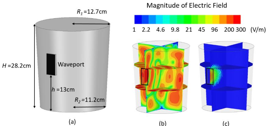
**Fig 2.** Simulated magnitude of the electric field for a single waveguide port excitation of a cavity completely filled with various materials. (a) Simulated cavity with dimensions labeled. (b) Cavity filed with food mixture  $\epsilon_r = 42$  and  $\tan\delta = .3$ , and (c) Cavity filled with LDPE and polystyrene  $\epsilon_r = 2.25$  and  $\tan\delta = .0003$ . The field value is normalized to a 1W incident power at 2.45 GHz on waveguide port.
