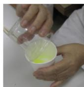
Add a portion of borax solution into laundry starch (polyvinyl alcohol) under stirring, the mixture gets hard. Add a bit of fluorescence produces shining slime
