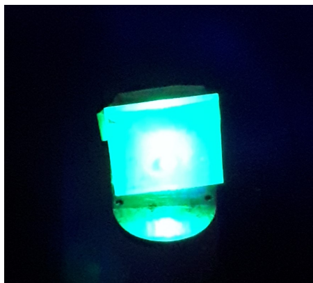
Figure 10: Photograph taken of the inner chamber of the PL equipment with the \text{MAPbBr}_{1.5}\text{Cl}_{1.5} sample being illuminated.
