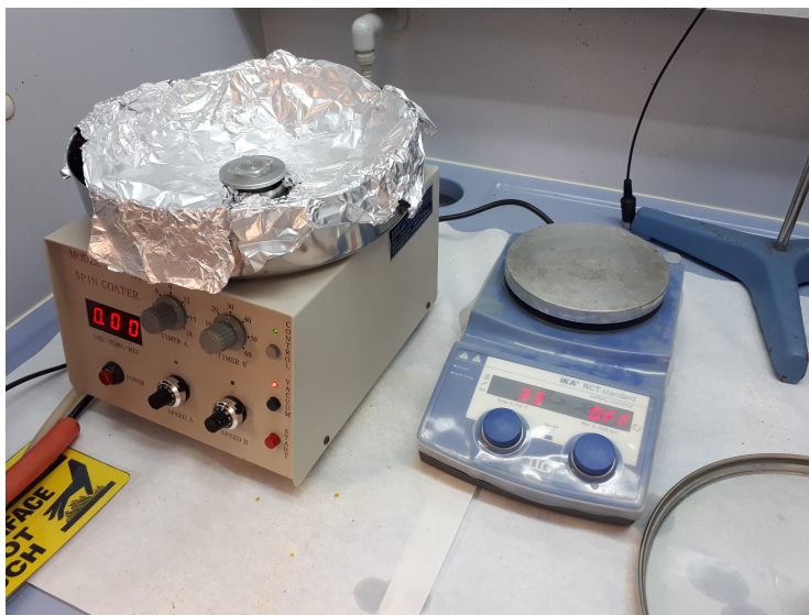
Figure 29: Set up for mesoporous layer spin-coating
