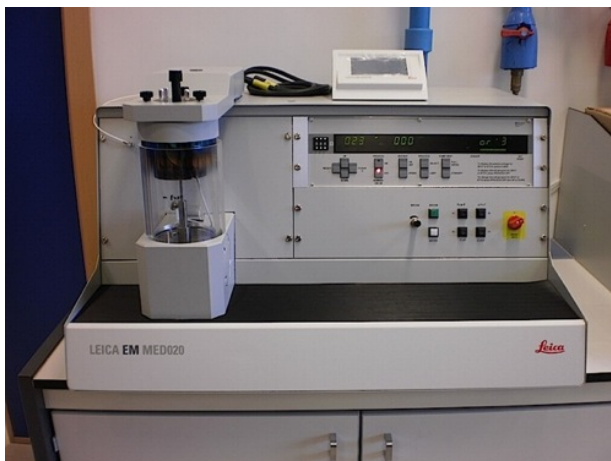
Figure 30: Set up for evaporation of gold contacts.
