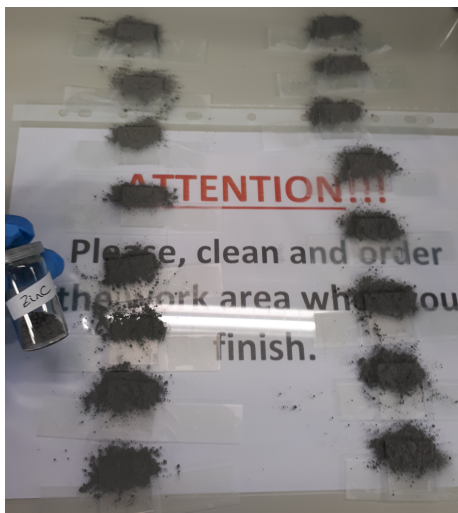
Figure 27: Applying Zinc for etching.
