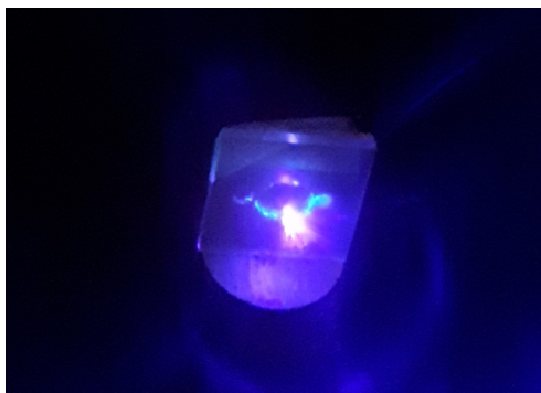
Figure 11: Photograph taken of the inner chamber of the PL equipment with the chlorine sample being illuminated.
