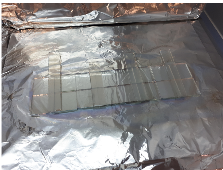
Figure 28: Set up for compact layer spray pyrolysis
