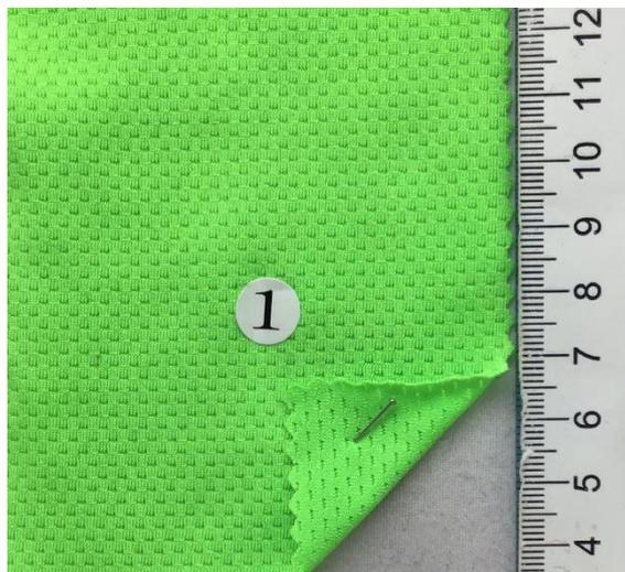
Figura 50: QL-017814 Forro Interior Poliéster + PU + Elastano
