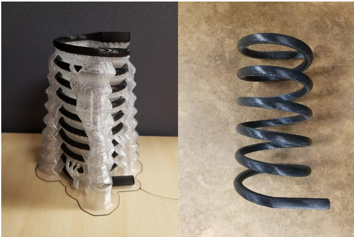
Figure 31: Helicoid with the tree-shaped support structure of the 3D printing and after removing the support structure
