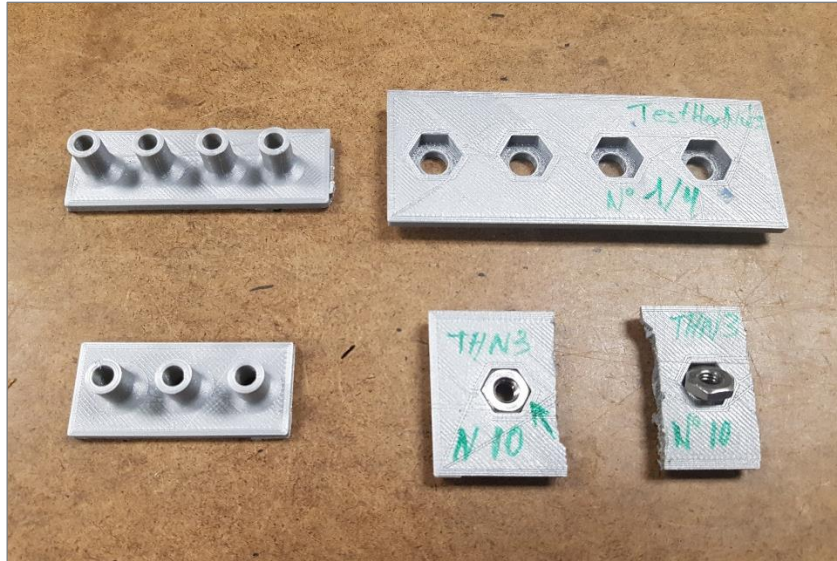
Figure 29: Support cylinders tests for the screws (on the left) and hexagonal holes tests for the nuts (on the right)
