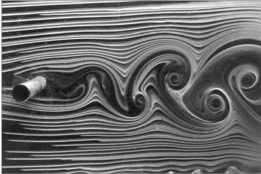
Figure 4: Experimental case of Vortex shedding in a cylindrical tube
