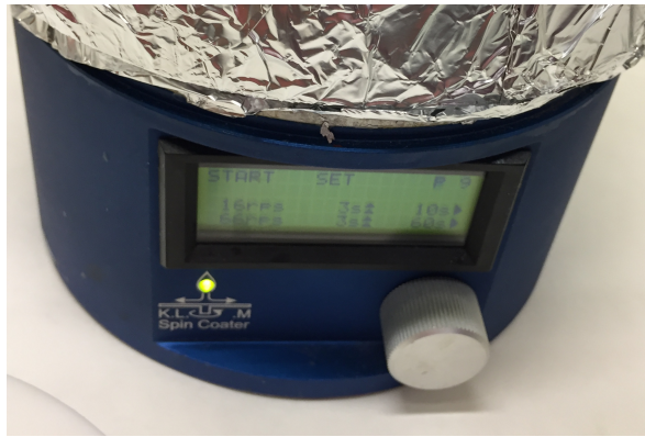
Figure 4.12: Spinner coater used for deposition of polyimide.
