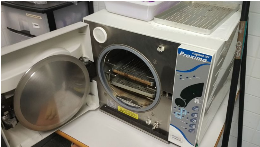
Figure 5.7: Instance of an autoclave for carrying out steam sterilization.
