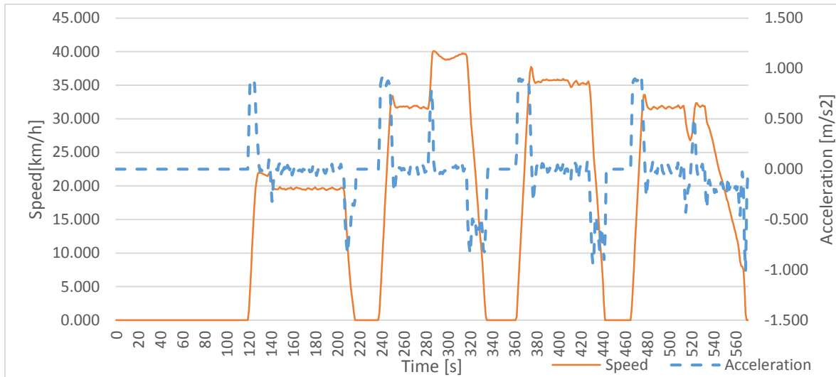
Figure 4. Speed (blue) and acceleration (orange) of the first trip between Marítim-Serrería and Alameda
