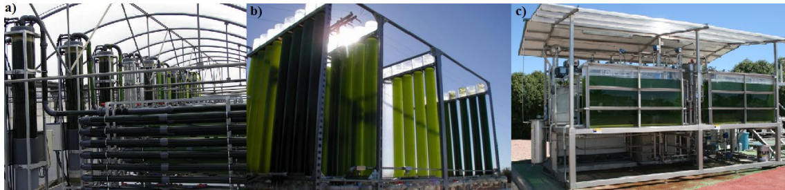
Figure I.4. Closed PBRs: a) Tubular PBRs (de Andrade et al., 2016); b) vertical columns (www.oilalgae.com); c) Flat-panel PBR.
