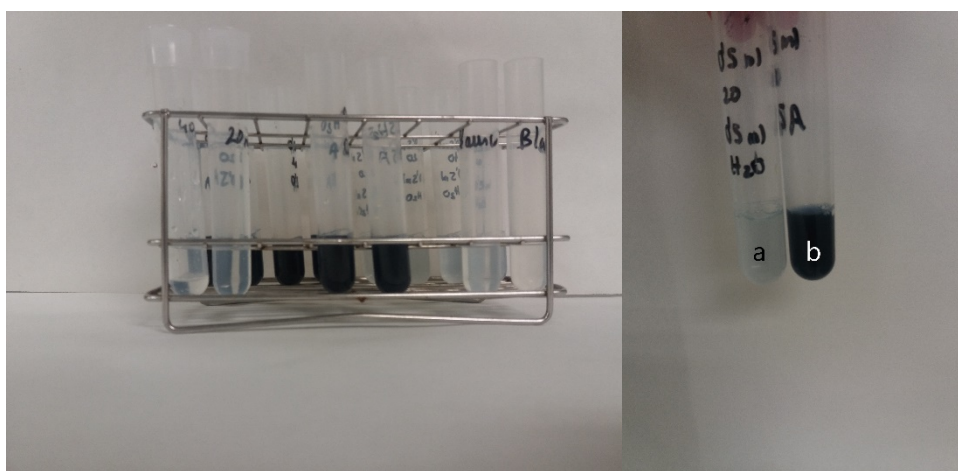
Figure XI.A.2: Lowry method modified by Peterson applied to samples with (b) and without ATU (a)
