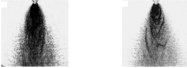
Figure 1.5: Data from Linne et al. [23] as an example of ballistic imaging results.
