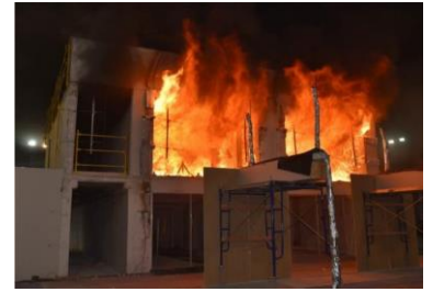
Fig.42: test de incendio a escala completa, XLam Australia Pty Ltd
