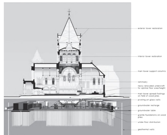
FIG. 13: The new design of the 4000 wooden piles submerged in water, routes all storm-water into drywells for dispersion back into the ground to maintain consistent groundwater levels and protect the integrity of the pilings. Source: Carroon, 2010, Sustainable Preservation: Greening Existing Buildings, p. 32).
