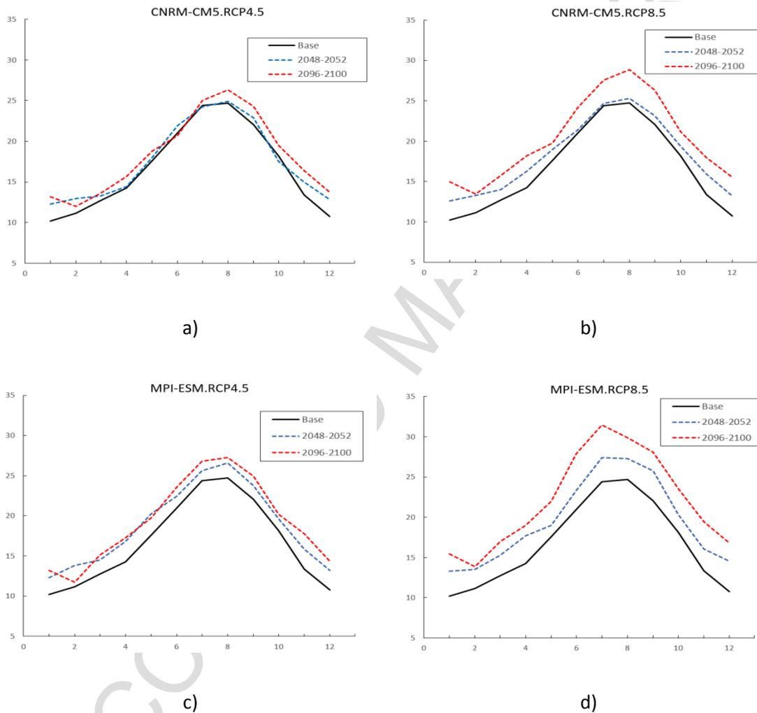
Figure 3. Monthly average dry bulb temperature (DBT) for the Base Scenario, in two periods: 2048-2052 and 2096-2100 under the following scenarios: a) CNRM-CM5 and RCP4.5; b) CNRM-CM5 and RCP8.5; c) MPI-ESM-LR and RCP4.5; d) MPI-ESM-LR scenario and RCP8.5.
