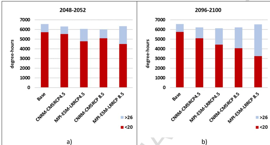
Figure 4. Number of heating (red) and cooling (blue) degree-hours in one year, using set-point temperatures (20 °C and 26 °C) for a) 2048-2052 and b) 2096-periods, in accordance with scenarios CNRM-CM5 and MPI-ESM-LR and the Representative Concentration Pathways RCP4.5 and RCP 8.5.
