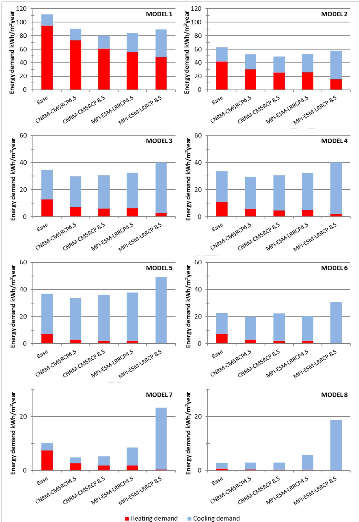
Figure 5. Annual energy demand for the Base Scenario and different models in a window of 2048 to 2052 in accordance with the following scenarios: CNRM-CM5 and RCP4.5; CNRM-CM5 and RCP8.5; MPI-ESM-LR and RCP4.5; and MPI-ESM-LR and RCP8.5.
