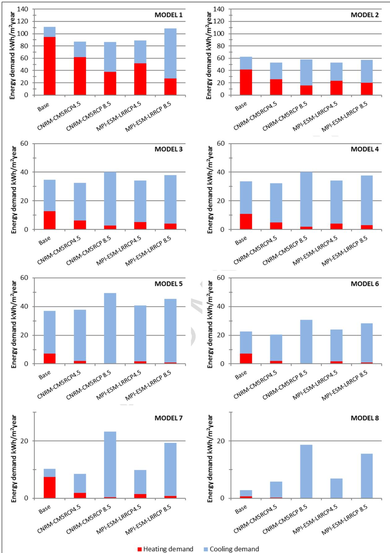
Figure 6. Annual energy demand for the different models in 2096-2100 period, for the Base Scenario and for the following scenarios: CNRM-CM5 and RCP4.5; CNRM-CM5 and RCP8.5; MPI-ESM-LR and RCP4.5; and MPI-ESM-LR and RCP8.5.
