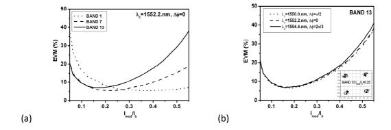
Fig. 6: EVM calculations as a function of the modulation ratio for: (a) three MB-OFDM bands, i.e. bands 1, 7 and 13, at  $\lambda_2$ =1552.2 nm for different modulation ratios; and (b) MB-OFDM band 13 for three different wavelengths through phase tuning.
