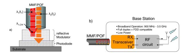
Fig. 9: (a) transceiver schematic drawing (reflective modulator sensitive for  $\lambda_1$ , quasi-transparent for  $\lambda_2$ ), (b) BS architecture for single fibre WDM MMF link in DAS.
