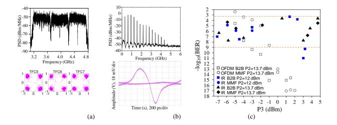
Fig. 11: (a) OFDM-UWB generated signal spectrum and constellations, (b) IR-UWB generated monocycles time electrical spectrum and time signal, (c) Performance comparison of OFDM and IR UWB RoMMF distribution in terms of BER vs. optical power injected into the fibre (P3) and different launch power levels (P2).
