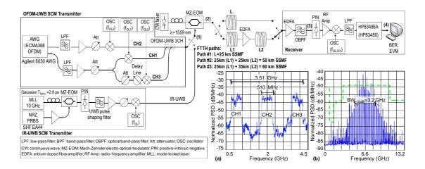
Figure 1: Experimental setup for UWB RoF distribution for FTTH. Generated signal spectrum for: (a) OFDM-UWB, (b) IR-UWB.
