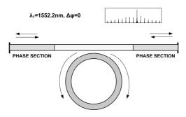
Fig. 5: Planar view of proposed microring laser transmitter with added phase sections enabling multi-wavelength operation.
