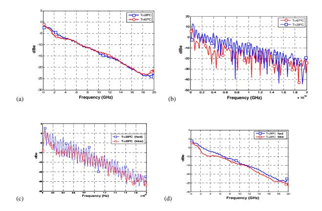
Fig.12: (a) Experimental frequency response of the MMF fibre link at  $T=28^{\circ}$ C and  $T=67^{\circ}$ C for L=3050m and  $\lambda=1300$ nm with Avg=16. (b) Measurement of the frequency response of an L=3050m MMF fibre link at  $\lambda=1300$ nm for a single sweep, (c) Hysteresis of the MMF link at the environmental temperature for a single sweep. (d) Averaged hysteresis of the MMF link at the environmental temperature. Fwd: forwards; Bkw: backwards
