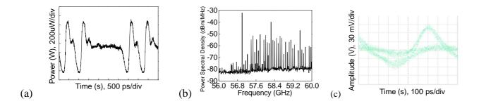
Fig. 4: (a) Optical baseband monocycles at point (1), (b) RF spectrum of the UWB signal at 57 GHz at point (2), (c) Eye diagram of demodulated monocycles at point (3) in Fig. 3.
