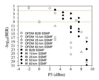
Figure 2: Performance comparison of OFDM and IR UWB RoF SMF distribution in terms of BER vs. received optical power for different FTTH SMF links.
