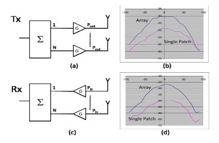
Fig. 7: a) Cloned transmitter array, b) Experimental 2×2 transmitter multiplicity advantage featuring additional 9dB gain, c) Cloned receiver array, d) Experimental 2×2 receiver array featuring a further 13dB gain, bringing overall link multiplicity advantage of 22 dB (c.f. theoretical gain of 24 dB).
