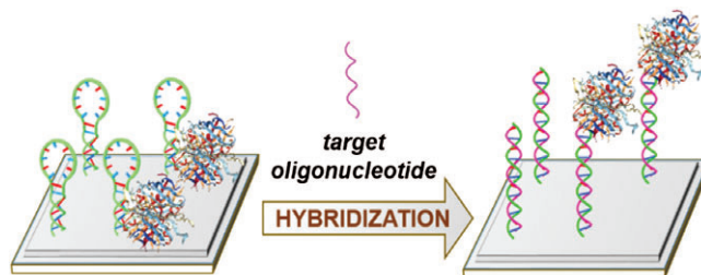
FIGURE 2 Scheme of the hybridization events for the streptavidin-free and the streptavidin-labeled molecular beacon (MB) probes being immobilized on the surface of a photonic structure
