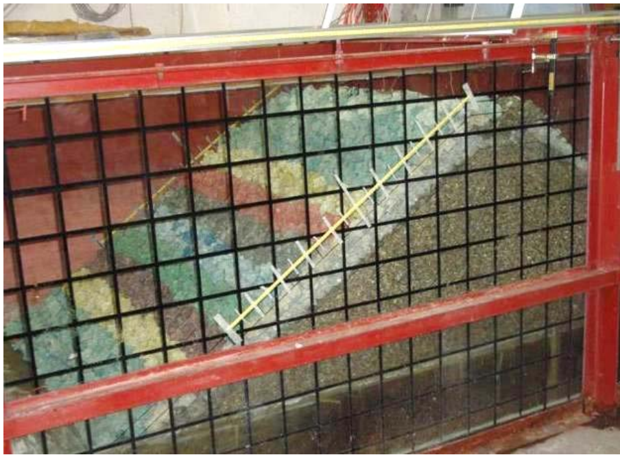
Figure 2. View of a double-layer Cubipod ® armored breakwater model without toe berm tested at the LPC-UPV.
