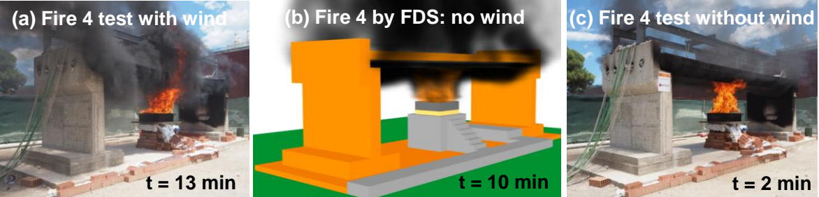
Figure 14. Different views of Fire 4 (a) Fire 4 test with wind (b) Fire 4 FDS model with no wind and (c) Fire 4 test with no wind.
