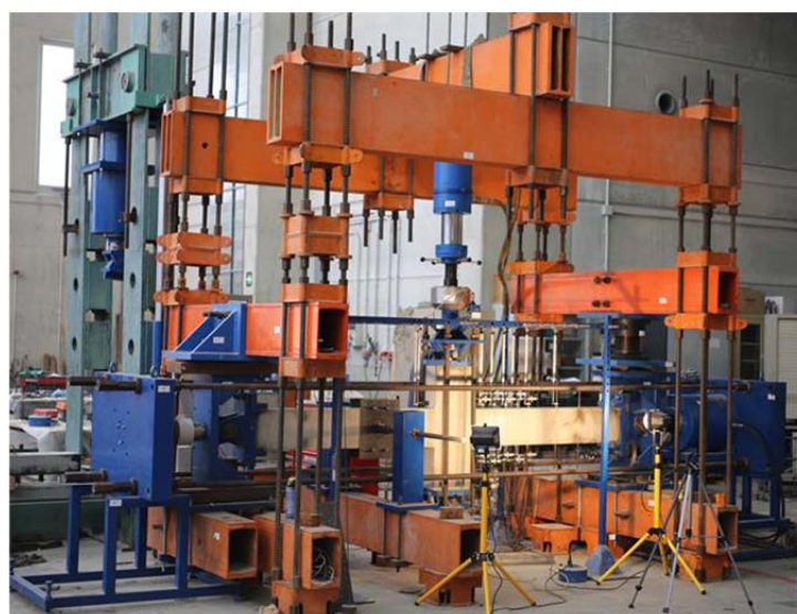
15 Figure 7. Beam-column element tested in the laboratory (Pereiro et al. [2]). 16
