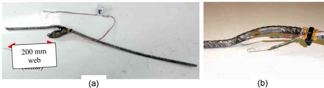
3 Figure 13: Final appearance of a flange transverse reinforcement, beam V1-0: (a) The 4 remaining longest part of a reinforcement that broke, approximately 200 mm over the web plus 5 450 mm corresponding to the flange at one-side; (b) Detail of the strain gauge location zone.
