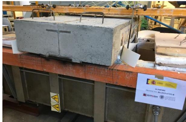
Fig. 8. Radiative furnace in ICITECH UPV testing facilities
