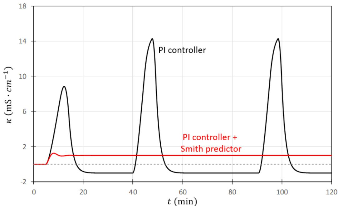
Figure 4: Comparison of the time evolution of the controlled variable (in deviation units) of a traditional PI controller versus a PI controller coupled with a Smith's predictor
