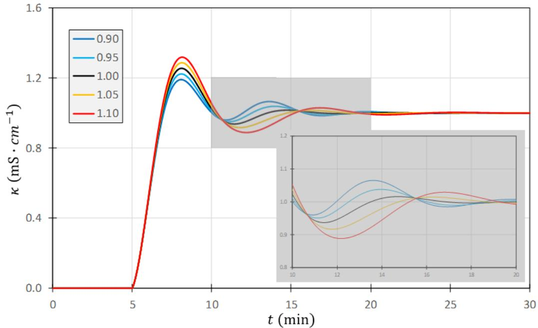
Figure 6: Effect of the error ( $e$ ) in the time constant of a non-ideal Smith's predictor ( $\tau' = e \cdot \tau$ ) on the time evolution of the controlled variable (in deviation units)
