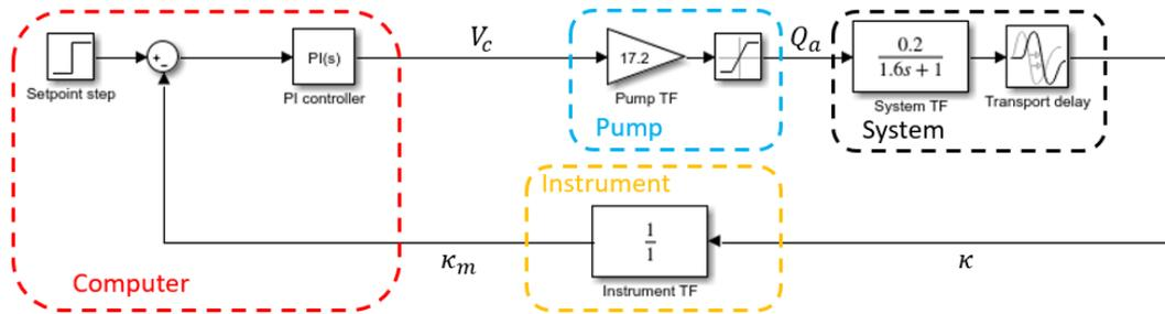
Figure 2: Simulink<sup>®</sup> model of the conductivity control system based on a PID controller
