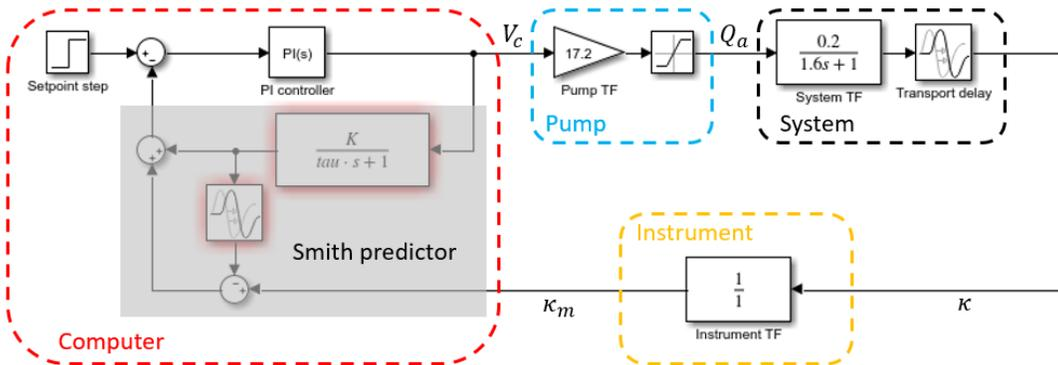
Figure 3: Simulink<sup>®</sup> model of the conductivity control system based on a PID controller coupled with a Smith's predictor
