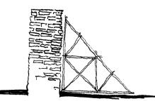
Fig. 15 the instillation of the buttress to support the falling wall
