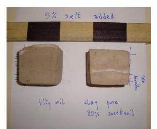
Fig. 22 Experiment of submerge the clay cube into salted water.
