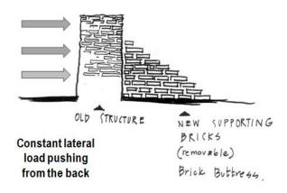
Fig. 2 The brick are being attacked by the salted water from the back, of the inclining wall
