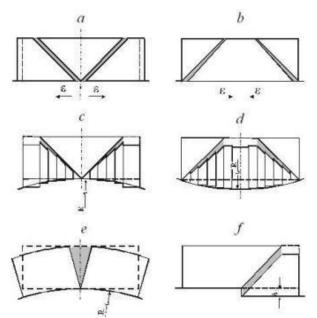
Fig. 7 The generalized structural deformations of the walls induced by: a – horizontal shear due to ground surface tension; b – horizontal shear due to the ground surface compression; c – vertical shear due to the curvature of convexity; d – vertical shear due to the curvature of concavity; e – bending due to the curvature of convexity; f – vertical shear due to the formation
