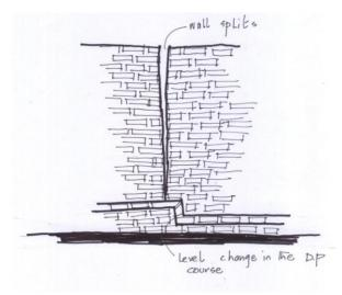
Fig.26 The elevation diagram of the wall
