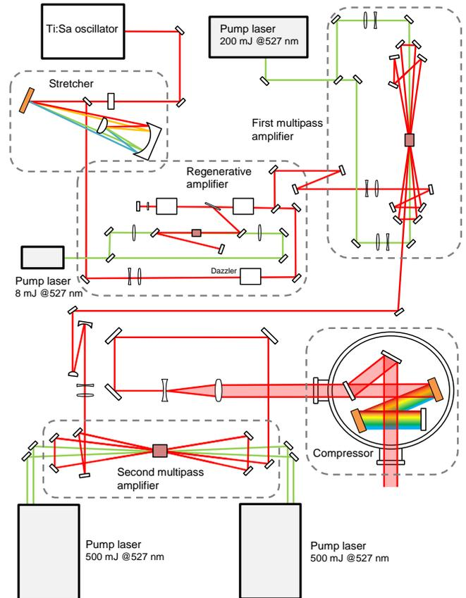
**Fig. 1** Scheme of the CPA Ti:Sa laser developed in the thesis. A pulse oscillator sends a beam of a few femtoseconds that is stretched in time in a pulse stretcher. Then it enters a chain of amplification that starts with a regenerative amplifier that is followed by a first multipass amplifier and ends with a second multipass amplifier. The CPA chain ends with a compressor installed in a vacuum chamber.
