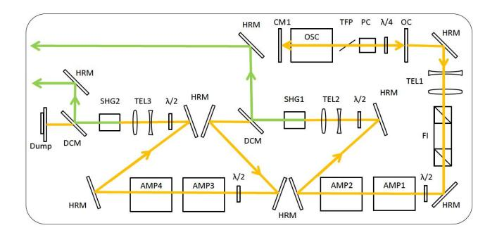
Fig. 2 Scheme of a MOPA Nd:YLF laser with 5 pumping heads (OSC, AMP1-4). CM1 and OC are the two mirrors that comprise the oscillator, along with a pumping heads, a thin film polarizer (TFP), a Pockels cell (PC) and a quarter waveplate  $\lambda/4$ . The setup includes a Faraday Isolator (FI) and three telescopes (TEL1-3). (SHG1&2) represent non-linear crystals for second harmonic conversion. There are two dichroic mirrors (DCM1&2) and a beam dump. HRM are high reflectivity mirrors.
