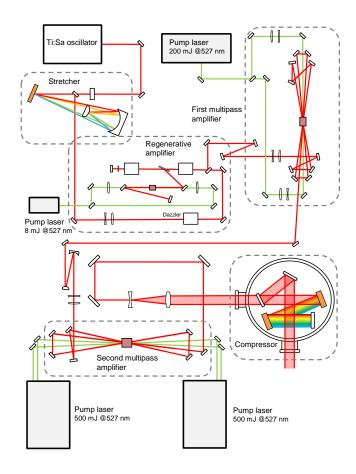
Fig. 1 Scheme of the CPA Ti:Sa laser developed in the thesis. A pulse oscillator sends a beam of a few femtoseconds that is stretched in time in a pulse stretcher. Then it enters a chain of amplification that starts with a regenerative amplifier that is followed by a first multipass amplifier and ends with a second multipass amplifier. The CPA chain ends with a compressor installed in a vacuum chamber.
