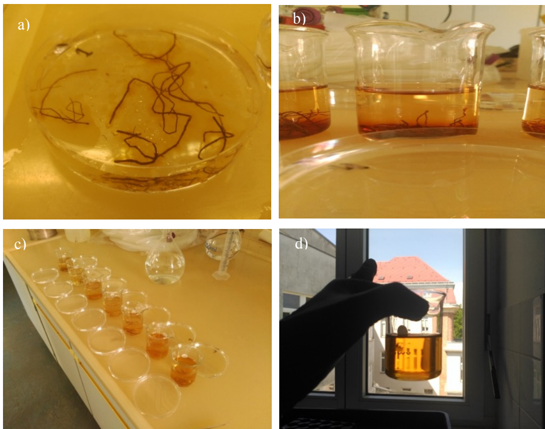
Figure 9. Bleaching process. Testing roots (a); pigments coming out (a, b and c), remaining H_2O_2 solution with pigments (d)
