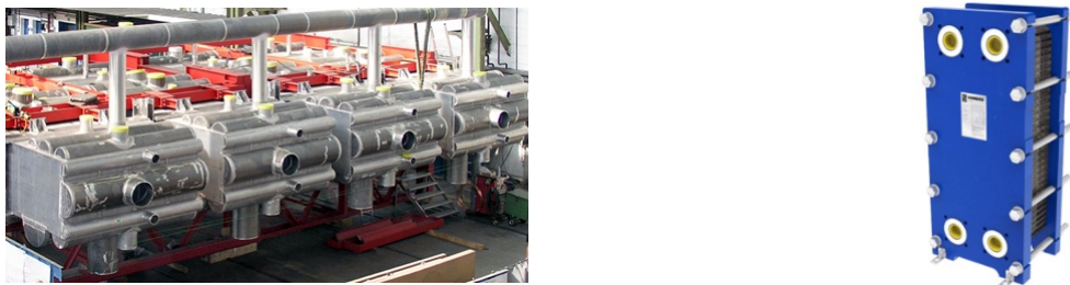
Figure 5: Plate-finned HEX designed by Linde AG (left) and welded plates HEX designed by Danfoss (right) [14]-[15].
