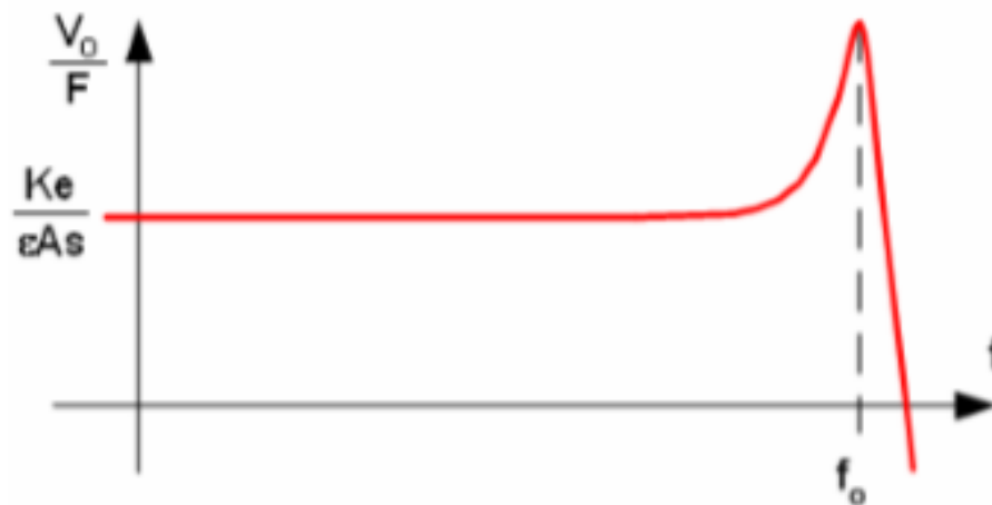
Figure 3.14: Transfer function of the output voltage of the sensor
