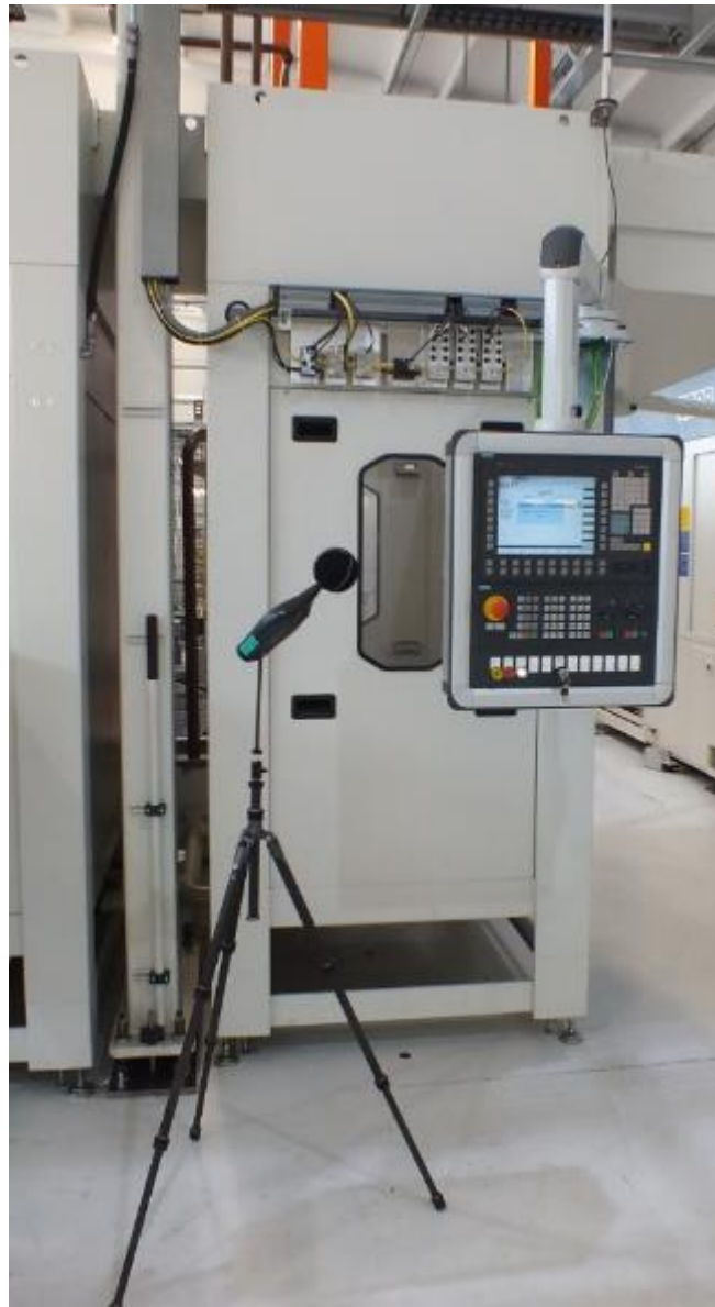
Figure 5-Measurement of the reverberation time
