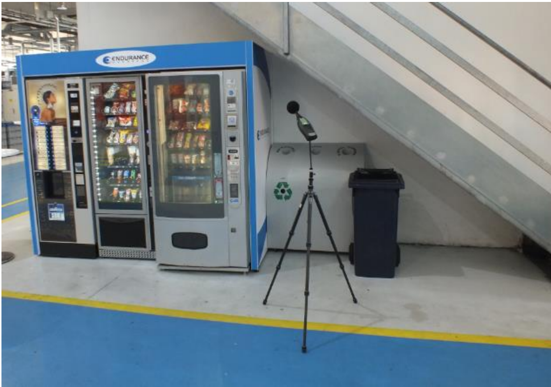
Figure 4- Location of the sound level meter to carry out measurements
