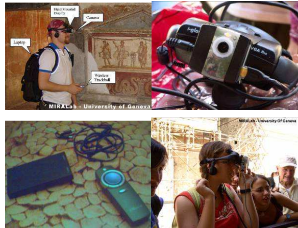
Fig. 9. The Mobile AR-Life simulator system (top left). The previously shown laptop is inserted in the backpack for the run phase. The IEEE1394 camera is attached on the i-glasses (top right) and a wireless trackball allows for interaction with the MR application (bottom left). The custom splitter cable (bottom left) allows for the i-glasses light lithium rechargeable battery to power both the HMD and the firewire camera (since in laptops the firewire port does not provide power). Thus true mobility is achieved surpassing existing car battery custom made heavier solutions [5]. More visitors have tried and tested on the site the AR-Life system (bottom right).
