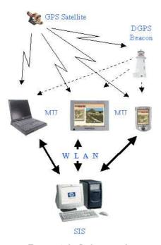
Figure 1. ArcheoGuide system architecture
