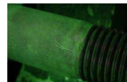
Fig. 5.40. Fluorescent, wet particle method ( https://goo.gl/79PNQo )
