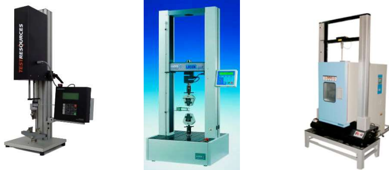
Fig. 1.22. a) Electromechanical universal test machine ( https://goo.gl/oAcX4D ); b) Universal test machine / single column / double column / numeral control. AMETK ( https://goo.gl/38LhLM ); c) Universal Testing Machine With Environmental Chamber. Gester ( https://goo.gl/j6gUAR )
