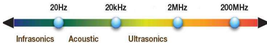
Fig. 5.12. Range of frequencies. Homemade and https://goo.gl/Rg9TF7
