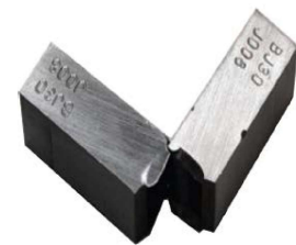
Fig. 6.9. Charpy pendulum cracked specimen (Ibertest)
