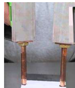
Fig. 1.18. Magnetization by contact tips. ( https://goo.gl/Dp2vbi )
