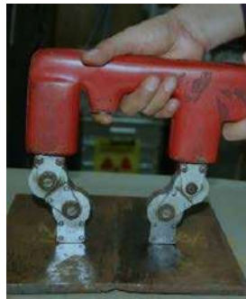
Fig. 1.18. Magnetization of a piece with the yoke (Goñi Córdoba, 2015, pág. 78)
