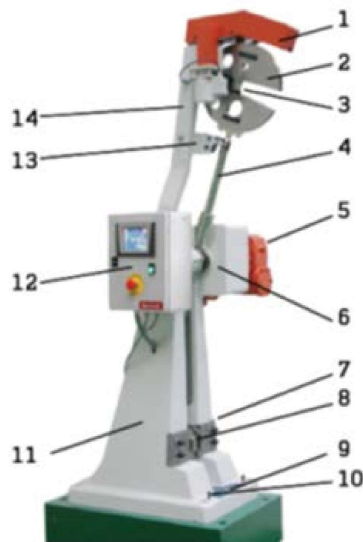
Fig. 1.26. Pendulum impact test IBERTEST Serie PIB ( https://goo.gl/ERK5v1 )
