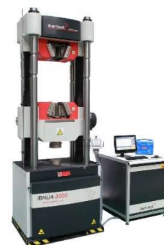
Fig. 6.6. Universal testing device Ibertest IBMU4 ( https://goo.gl/HKg162 )
