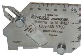
Fig. 1.6. Calibrator Bridge Cam ( https://goo.gl/ovqFEc )
