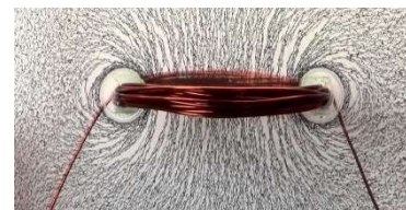
Fig. 5.37. Longitudinal magnetization coi. ( https://goo.gl/HKLBb9 )
