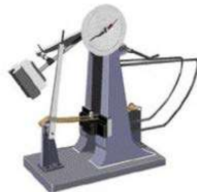
Fig. 6.8. Charpy testing. ( https://goo.gl/GFyRyF )
