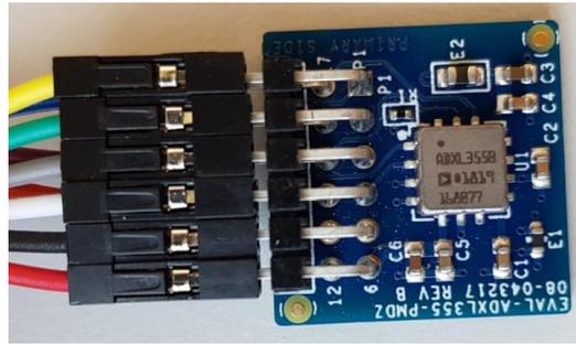
Figure 3: Accelerometer ADXL355
