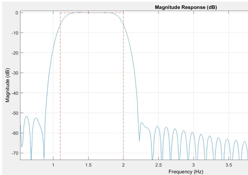
Figure 25: Algorithm 1– bandpass filter
