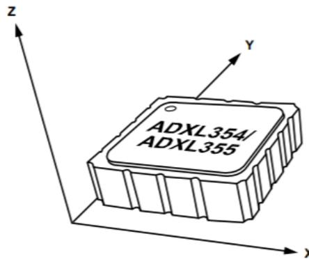
Figure 5: Axes of Acceleration [4]
