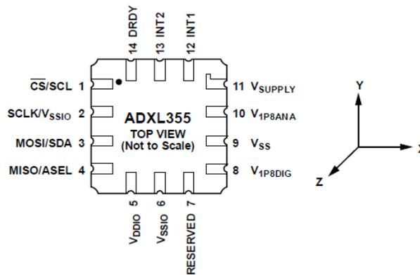
Figure 4: Accelerometer - Pin Configuration [4]
