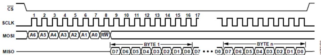
Figure 8: SPI Protocol – Multibyte Read [4]
