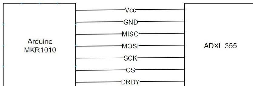
*Figure 12: Scheme of connection between microcontroller and accelerometer*
