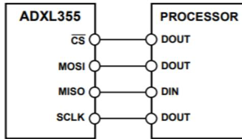
Figure 7: 4-wire SPI connection [4]
