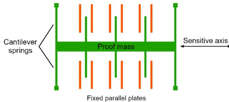
Figure 2: MEMS principle of operation
