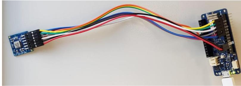
*Figure 13: pin connection between accelerometer and microcontroller*
