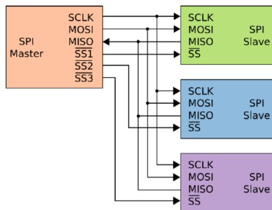
Figure 6: SPI master slave communication protocol
