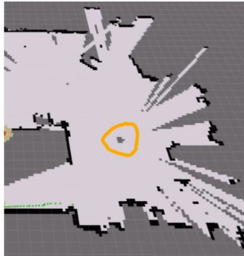
Figure 80. Filtered map with a non-adjacent detected obstacle.
