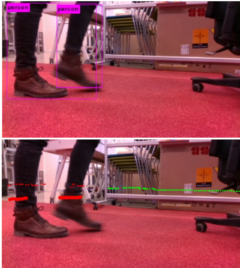
Figure 73. Resulting included (in green) and excluded (in red) pointcloud data printed directly to the camera data from the laser scanner.
