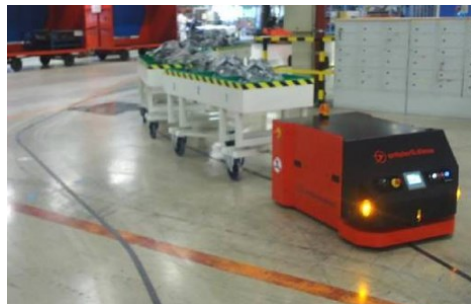
AGV navigation system based on guided tapes. [6]
