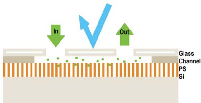
Fig. 4. Schematic view of the PS structure attached to the substrate together with the microfluidic cell. The flow path is illustrated with green dots. The blue arrow represents the place where reflectance was measured. Note that the inlet and outlet are placed in the glass instead of in the PDMS (which is not used in this setup).
