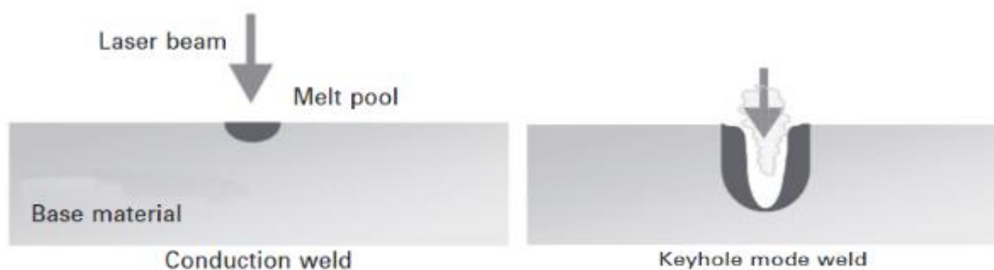
Figure 5. Comparison between keyhole and conduction (Katayama, 2013)
