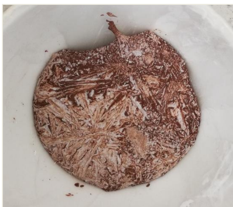
Figure 88. Aspect of the sample 2 of GP3-Fine (24 th curing day).
