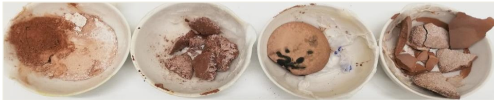
Figure 50. From left to right, aspect of the sample 1, 2, 3 and 4 of GP3-Fine after crushing (physical stability test). Sample 1, 2 and 4 on the 31th curing day; sample 3 on the 34th curing day (Study 2).
