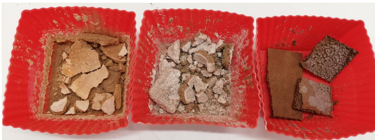
Figure 26. From left to right, aspect of the samples 1, 2 and 3 of the GP3-Granulated after crushing (physical stability test; 36 th curing day).
