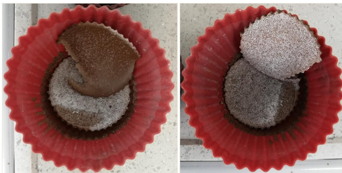
Figure 57. Aspect of the sample 3 of GP6-Granulated on the 28 th curing day.
