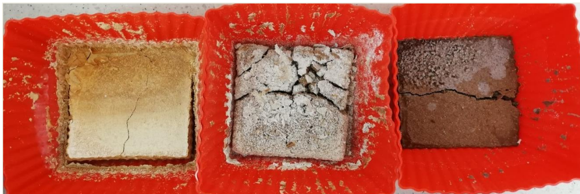
Figure 22. From left to right, aspect of the samples 1, 2 and 3 of the GP3-Granulated (34 th curing day).
