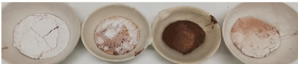
Figure 100. From left to right, aspect of the sample 1, 2, 3 and 4 of GP4 before crushing (physical stability test). Sample 1, 2 and 4 on the 31 th curing day; sample 3 on the 33 th curing day (Study 2).
