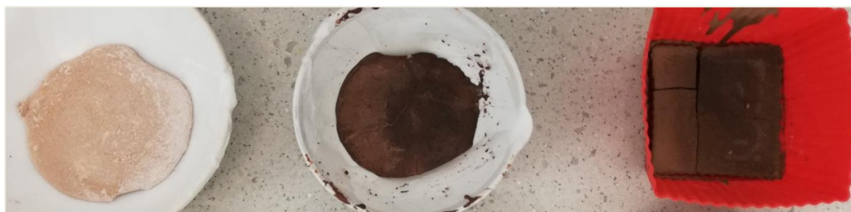
Figure 114. From left to right, aspect of the sample 1, 2 and 3 of GP6-Fine. Sample 1 on the 29 th curing day; sample 2 on the 32 nd curing day; sample 3 on the 35 th curing day (Study 2).
