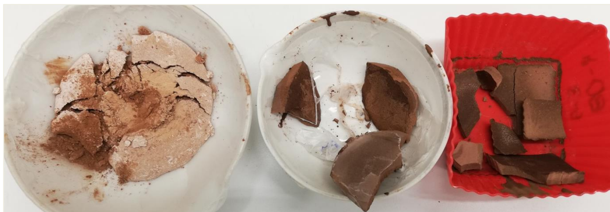
Figure 115. From left to right, aspect of the sample 1, 2 and 3 of GP6-Fine after crushing (physical stability test). Sample 1 on the 31 th curing day; sample 2 on the 34 th curing day; sample 3 on the 37 th curing day (Study 2).
