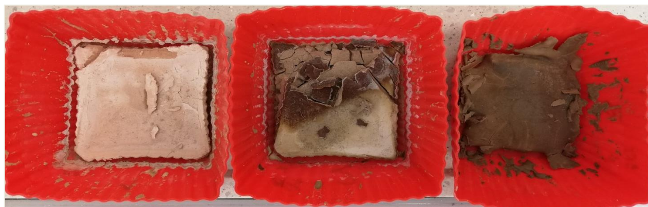
Figure 34. From left to right, aspect of the samples 1, 2 and 3 of the GP3-Fine (29 th curing day).
