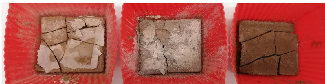
Figure 6. From left to right, aspect of the samples 1, 2 and 3 of the GP2 (12 th curing day).
