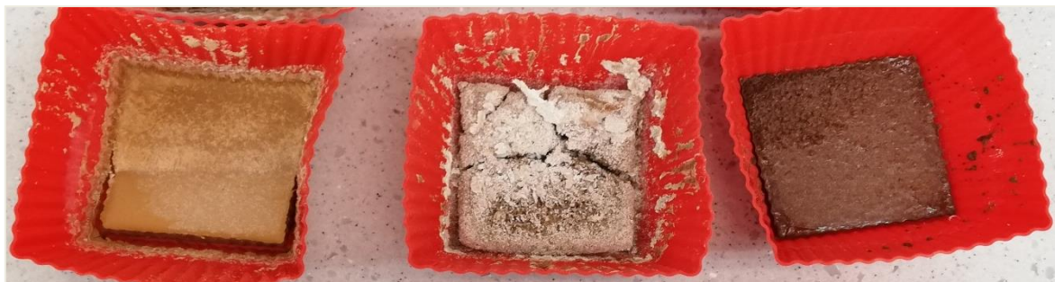
Figure 16. From left to right, aspect of the samples 1, 2 and 3 of the GP3-Granulated after being one day curing.
