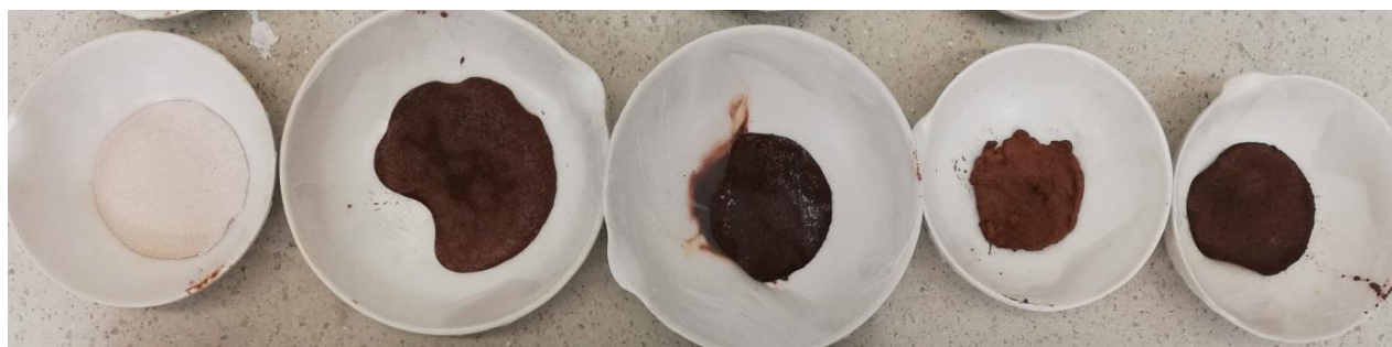
Figure 80. From left to right, aspect of the sample 1, 2, 3, 4 and 5 of GP3-Granulated (21 th curing day). (Study 2).
