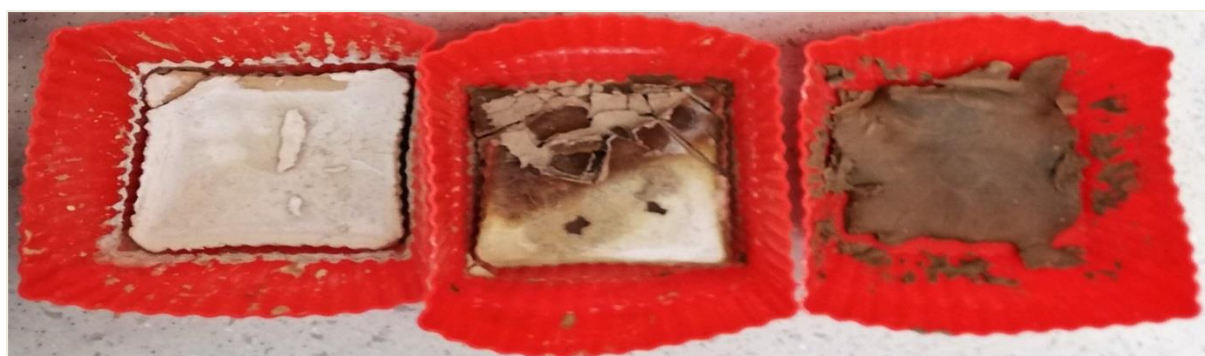
Figure 32. From left to right, aspect of the samples 1, 2 and 3 of the GP3-Fine (8 th curing day).
