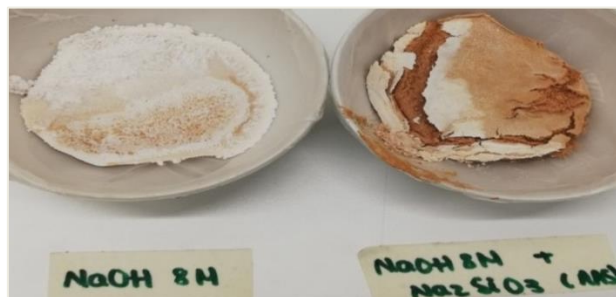
Figure 62. Aspect of the Jarosite Study 3-2 geopolymer on the 13th curing day.
