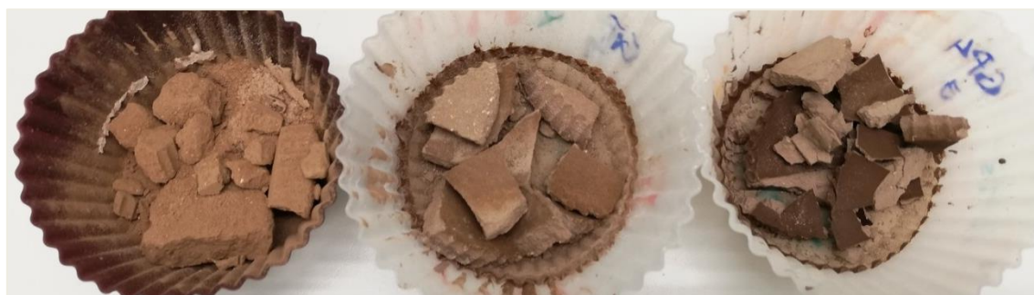
Figure 48. From left to right, aspect of the samples 1, 2 and 3 of the GP4 after crushing (physical stability test; 35 th curing day).
