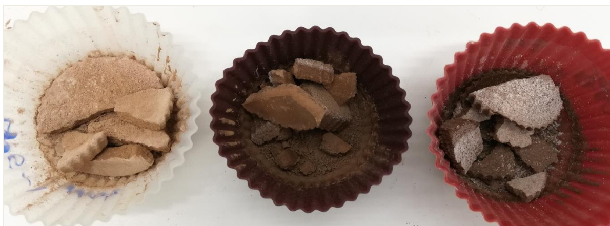
Figure 60. From left to right, aspect of the sample 1, 2 and 3 of GP6-Granulated after crushing (physical stability test). Samples 1 and 2 on the 34 th curing day. Sample 3 on the 35 th curing day.
