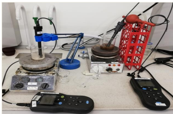
Figure 17. Experimental set-up for adsorption experiments.
