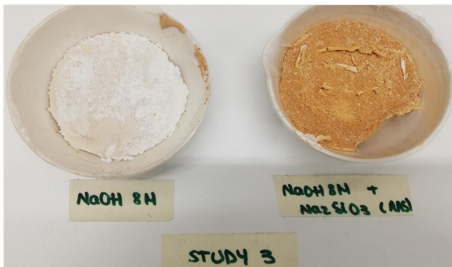
Figure 121. Aspect of the Jarosite Study 3-1 geopolymer on the 8 th curing day.
