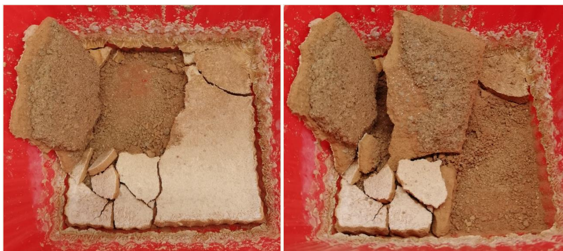
Figure 24. Aspect of the sample 1 of GP3-Granulated. Geopolymer no homogeneous (36 th curing day).
