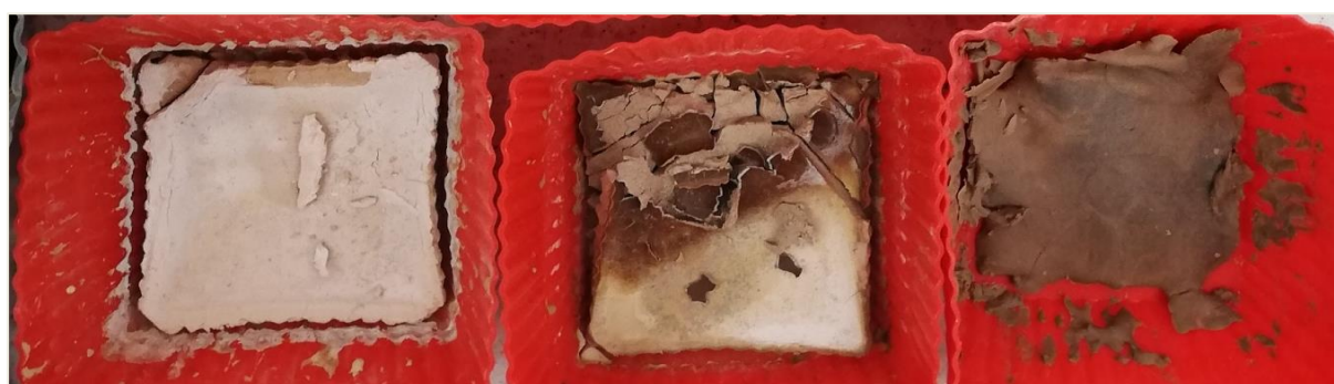
Figure 33. From left to right, aspect of the samples 1, 2 and 3 of the GP3-Fine (12 th curing day).
