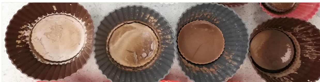
Figure 66. From left to right, aspect of the sample 1, 2, 2' and 3 of GP6-Fine. Sample 1, 2 and 2' on the 7 th curing day. Sample 3 on the 8 th curing day.
