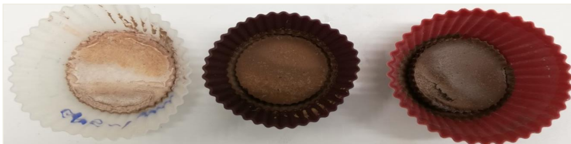
Figure 51. From left to right, aspect of the sample 1, 2 and 3 of GP6-Granulated. Samples 1 and 2 on the 3 rd curing day. Sample 3 on the 4 th curing day.
