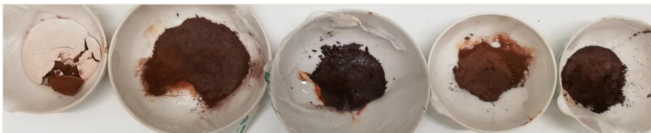
Figure 82. From left to right, aspect of the sample 1, 2, 3, 4 and 5 of GP3-Granulated after crushing (28 th curing day). (Study 2).
