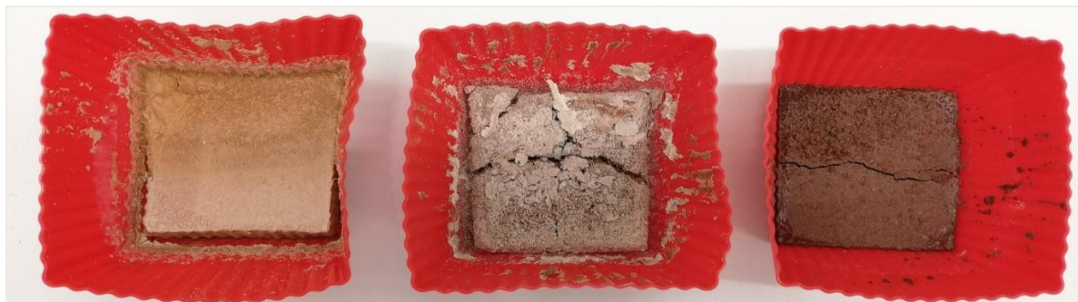
Figure 18. From left to right, aspect of the samples 1, 2 and 3 of the GP3-Granulated (6 th curing day).
