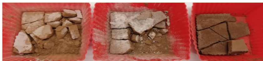
Figure 25. From left to right, aspect of the samples 1, 2 and 3 of the GP2 after crushing (physical stability test; 42th curing day).
