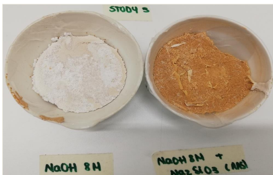
Figure 122. Aspect of the Jarosite Study 3-1 geopolymer on the 21 th curing day.
