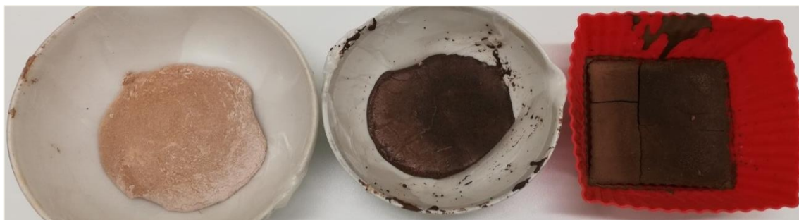
Figure 113. From left to right, aspect of the sample 1, 2 and 3 of GP6-Fine. Sample 1 on the 21 th curing day; sample 2 on the 24 th curing day; sample 3 on the 27 th curing day (Study 2).
