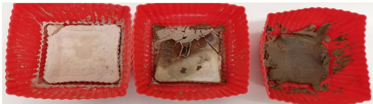
Figure 31. From left to right, aspect of the samples 1, 2 and 3 of the GP3-Fine (6 th curing day).
