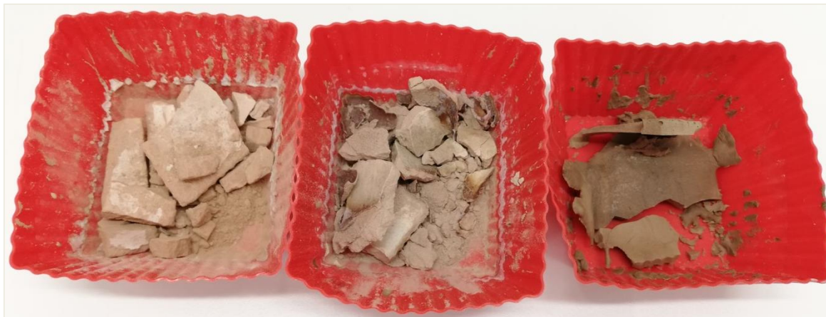
Figure 38. From left to right, aspect of the samples 1, 2 and 3 of the GP3-Fine after crushing (physical stability test; 36 th curing day).
