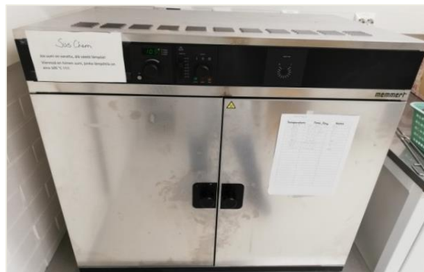
Figure 12. Drying laboratory oven at 105°C.
