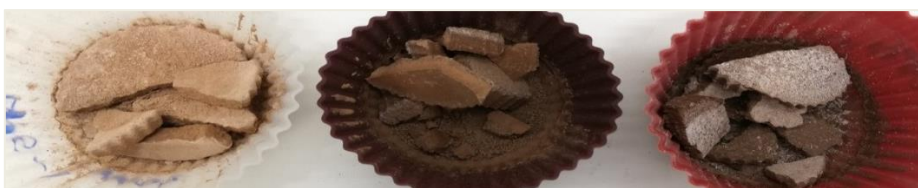
Figure 37. From left to right, aspect of the sample 1, 2 and 3 of GP6-Granulated after crushing (physical stability test). Samples 1 and 2 on the 34th curing day. Sample 3 on the 35th curing day.
