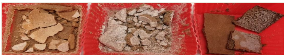
Figure 28. From left to right, aspect of the samples 1, 2 and 3 of the GP3-Granulated after crushing (physical stability test; 36th curing day).
