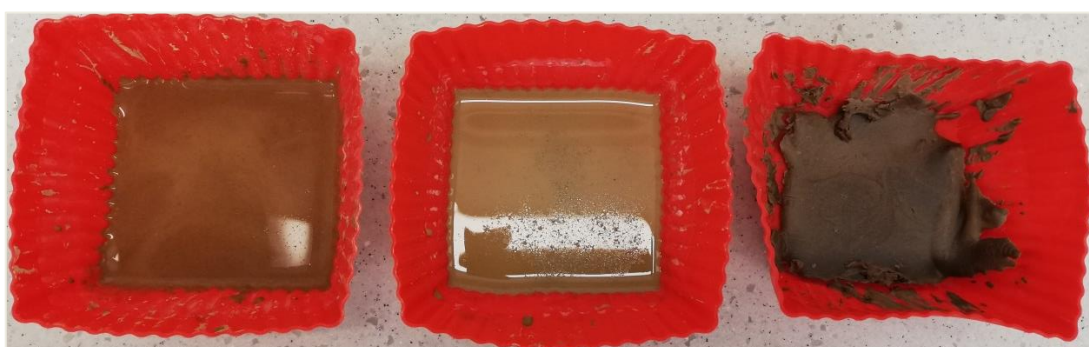
Figure 28. From left to right, aspect of the samples 1, 2 and 3 of the GP3-Fine. For the sample 1 and 2, aspect after being synthesized. For sample 3, aspect after 2 h of synthesis.
