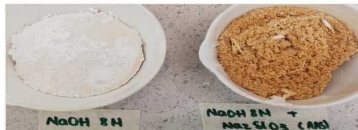
Figure 60. Aspect of the Jarosite Study 3-1 geopolymer on the 4th curing day.
