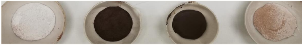
Figure 42. From left to right, aspect of the sample 1, 2, 3 and 4 of GP2. Sample 1, 2 and 4 after one curing day. Sample 3 on the 3rd curing day (Study 2).
