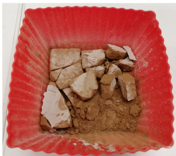
Figure 13. Enlarged photo of the aspect of the sample 1 of GP2 after crushed (physical stability test; 42 th curing day).
