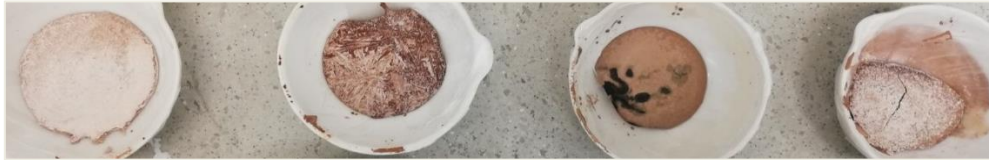
Figure 49. From left to right, aspect of the sample 1, 2, 3 and 4 of GP3-Fine. Sample 1, 2 and 4 on the 24th curing day; sample 3 on the 27th curing day (Study 2).
