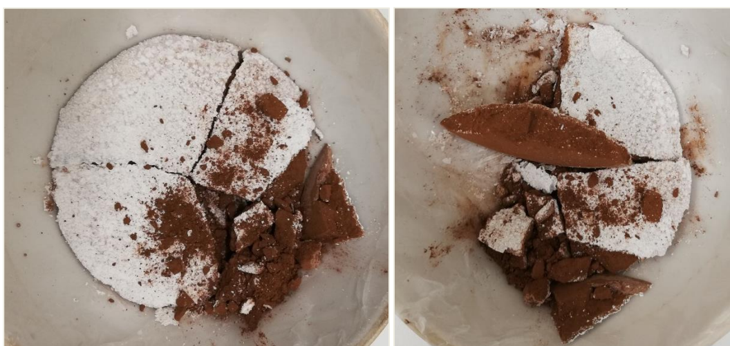
Figure 77. From left to right, aspect of the sample 1 and 2 of GP2 on the 29 th curing day after crushing (Study 2).
