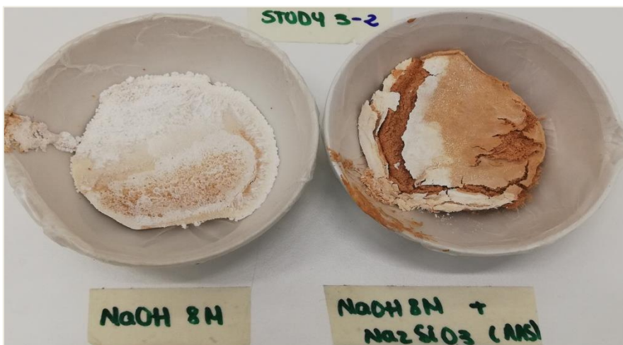
Figure 127. Aspect of the Jarosite Study 3-2 geopolymer on the 18 th curing day.
