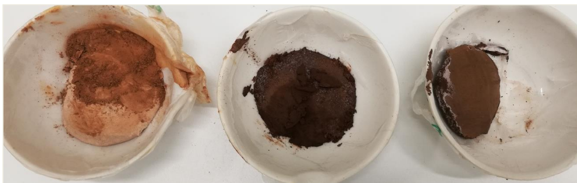
Figure 108. From left to right, aspect of the sample 1, 2 and 3 of GP6-Granulated after crushing (physical stability test) on the 29 th curing day (Study 2).
