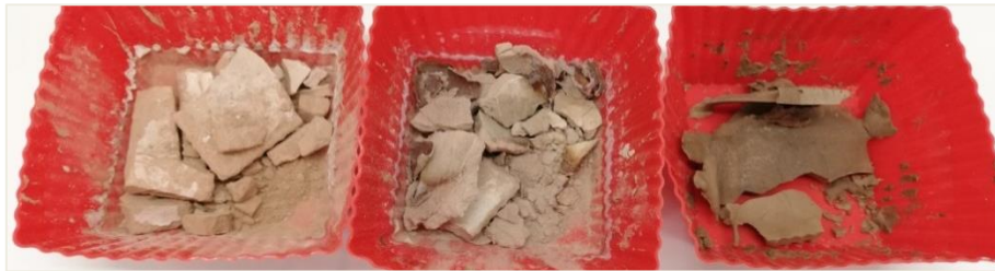
Figure 31. From left to right, aspect of the samples 1, 2 and 3 of the GP3-Fine after crushing (physical stability test; 36 th curing day).
