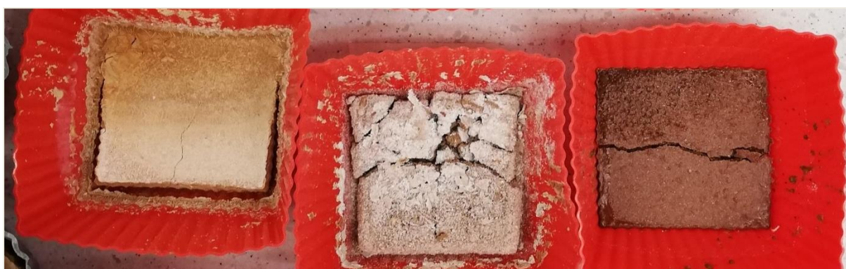
Figure 20. From left to right, aspect of the samples 1, 2 and 3 of the GP3-Granulated (12 th curing day).
