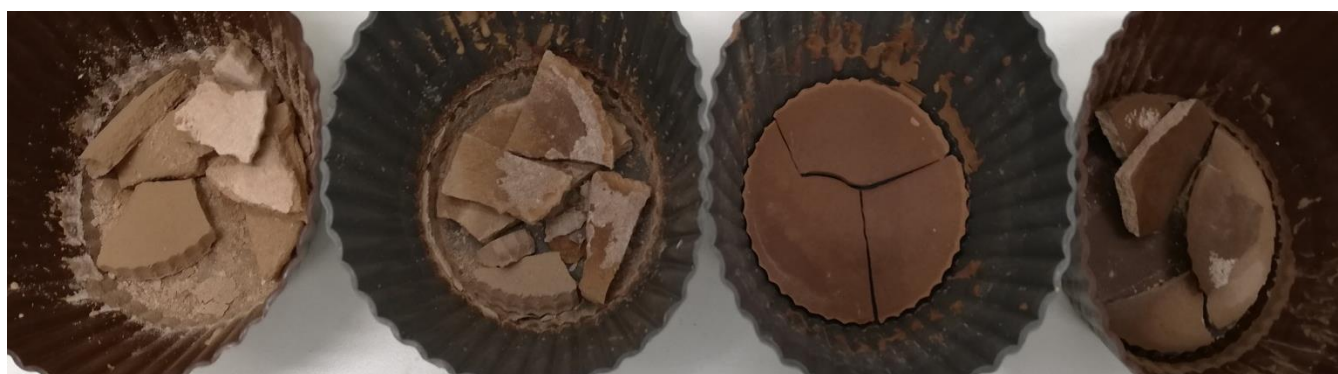
Figure 68. From left to right, aspect of the sample 1, 2, 2' and 3 of GP6-Fine after crushing (physical stability test). Sample 1 and 2 on the 33 th curing day. Sample 3 on the 35 th curing day.
