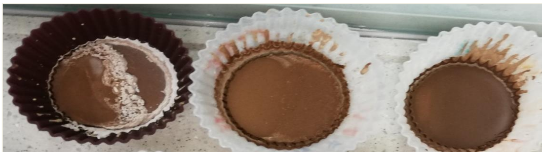
Figure 40. From left to right, aspect of the samples 1, 2 and 3 of the GP4 after one day curing.
