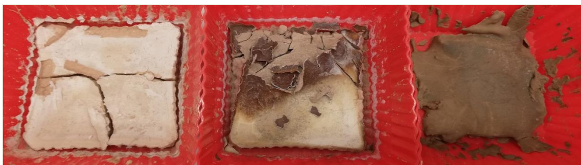
Figure 36. From left to right, aspect of the samples 1, 2 and 3 of the GP3-Fine (36 th curing day).
