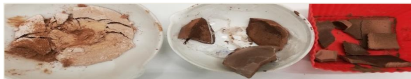
Figure 59. From left to right, aspect of the sample 1, 2 and 3 of GP6-Fine after crushing (physical stability test). Sample 1 on the 31 th curing day; sample 2 on the 34 th curing day; sample 3 on the 37 th curing day (Study 2).
