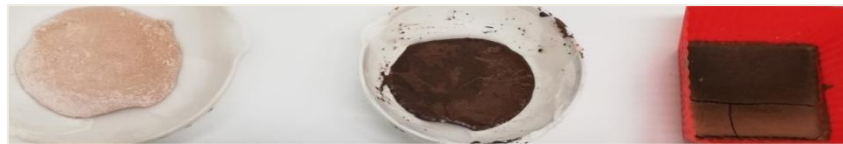
Figure 57. From left to right, aspect of the sample 1, 2 and 3 of GP6-Fine. Sample 1 once synthesized; sample 2 on the 3 rd curing day; sample 3 on the 6 th curing day (Study 2).
