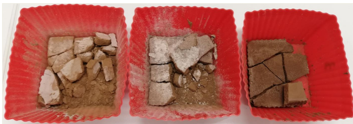
Figure 12. From left to right, aspect of the samples 1, 2 and 3 of the GP2 after crushing (physical stability test; 42 th curing day).
