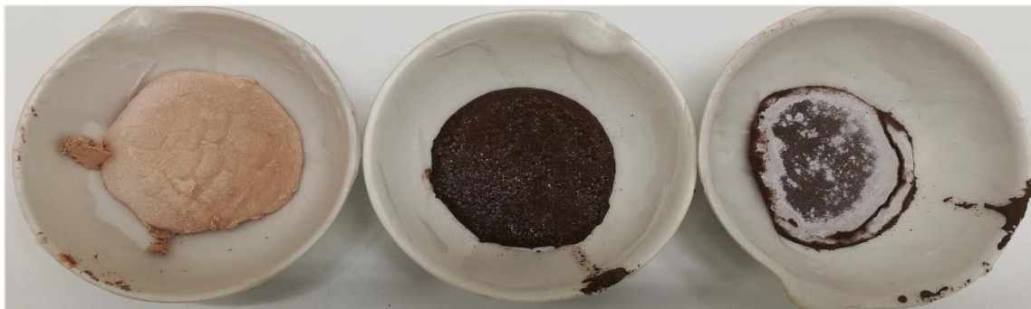
Figure 107. From left to right, aspect of the sample 1, 2 and 3 of GP6-Granulated before crushing (physical stability test) on the 29 th curing day (Study 2).
