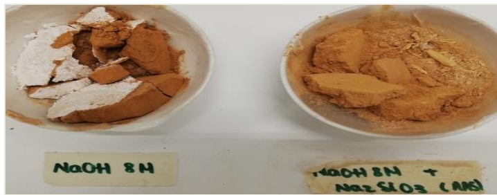
Figure 61. Aspect of the Jarosite Study 3-1 geopolymer on the 28th curing day after crushing (physical stability test).
