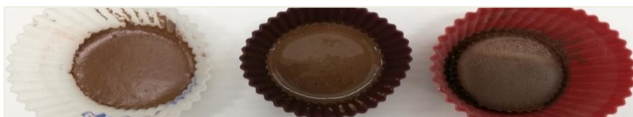
Figure 35. From left to right, aspect of the sample 1, 2 and 3 of GP6-Granulated. Samples 1 and 2 after synthesis. Sample 3 after 1 curing day.
