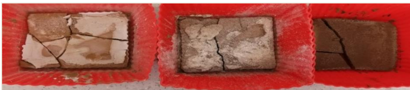
Figure 24. From left to right, aspect of the samples 1, 2 and 3 of the GP2 (3rd curing day).
