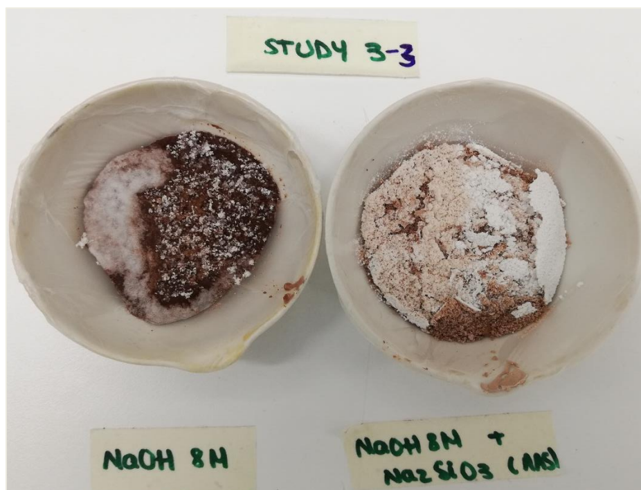
Figure 130. Aspect of the Jarosite Study 3-3 geopolymer on the 13 th curing day.
