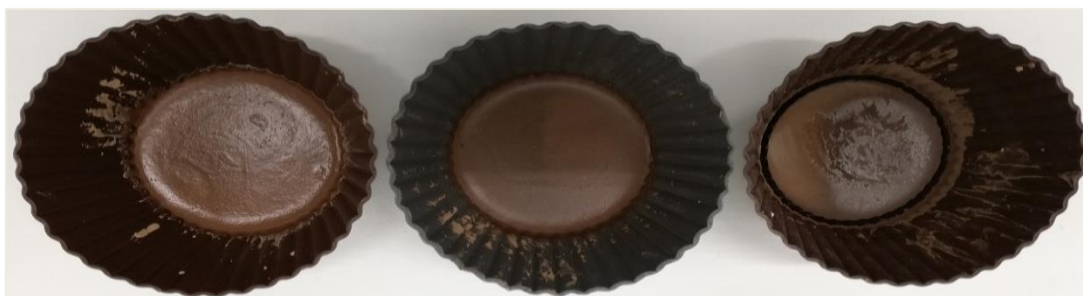
Figure 62. From left to right, aspect of the sample 1, 2 and 3 of GP6-Fine. Sample 1 and 2 after 1 h of the synthesis. Sample 3 after one day curing.
