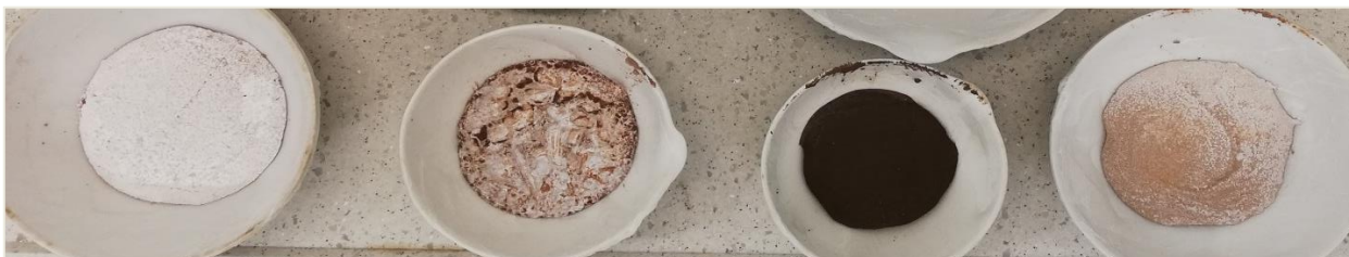
Figure 75. From left to right, aspect of the sample 1, 2, 3 and 4 of GP2. Sample 1, 2 and 4 on the 29 th curing day. Sample 3 on the 31 th curing day (Study 2).
