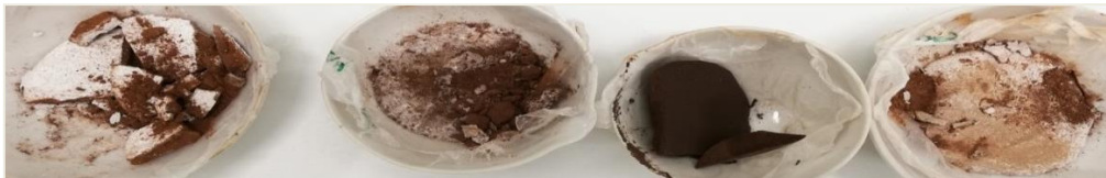
Figure 44. Aspect of the sample 1, 2, 3 and 4 of GP2 after crushing (physical stability test). Sample 1, 2 and 4 on the 29th curing day. Sample 3 on the 31th curing day (Study 2).
