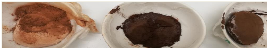
Figure 56. From left to right, aspect of the sample 1, 2 and 3 of GP6-Granulated after crushing (physical stability test) on the 29th curing day (Study 2).
