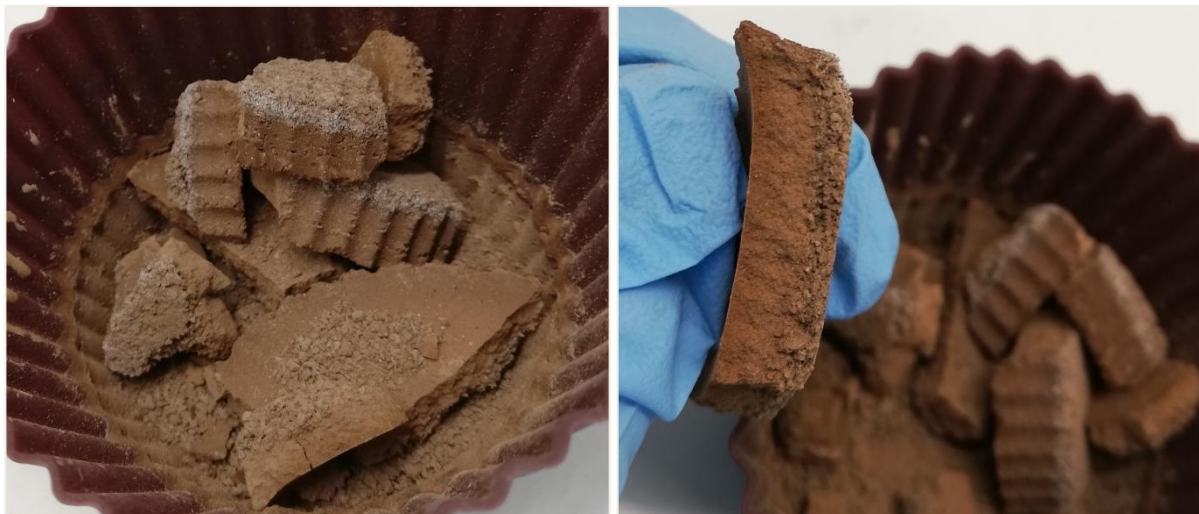
Figure 59. Aspect of sample 2 of GP6-Granulated after crushing (34 th curing day). Structure no uniform of the geopolymer.
