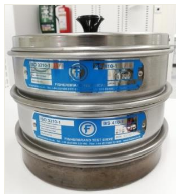
Figure 10. Mesh sieves from 1mm to 250 \mu m.
