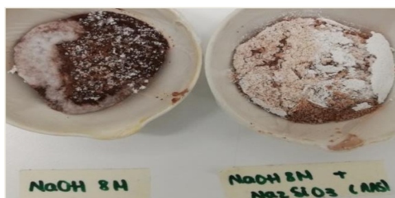
Figure 64. Aspect of the Jarosite Study 3-3 geopolymer on the 13th curing day.
