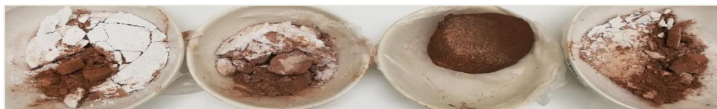
Figure 53. From left to right, aspect of the sample 1, 2, 3 and 4 of GP4 after crushing (physical stability test). Sample 1, 2 and 4 on the 31th curing day; sample 3 on the 33th curing day (Study 2).
