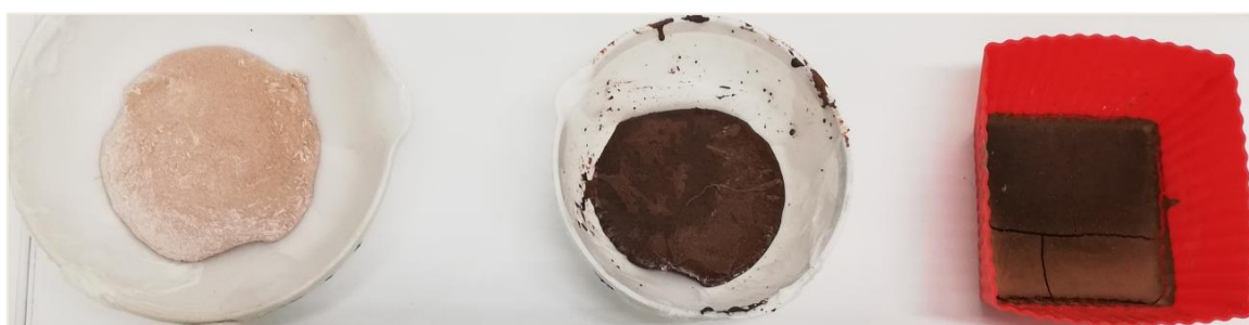
Figure 112. From left to right, aspect of the sample 1, 2 and 3 of GP6-Fine. Sample 1 once synthesized; sample 2 on the 3 rd curing day; sample 3 on the 6 th curing day (Study 2).
