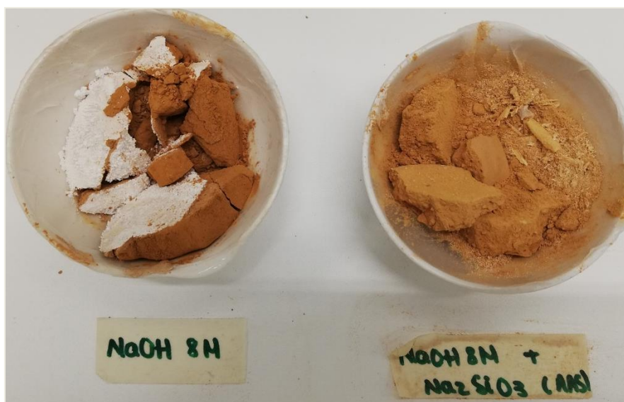
Figure 124. Aspect of the Jarosite Study 3-1 geopolymer on the 28 th curing day after crushing (physical stability test).
