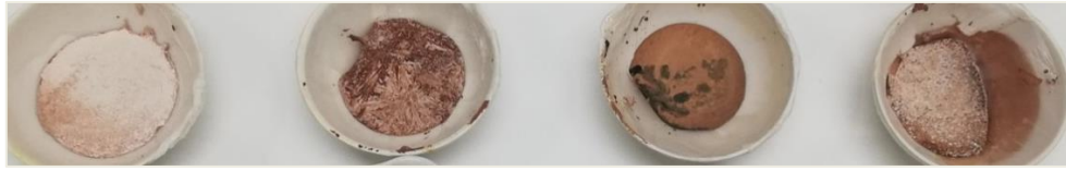
Figure 48. From left to right, aspect of the sample 1, 2, 3 and 4 of GP3-Fine once synthesized. Sample 3 on the 3rd curing day (Study 2).
