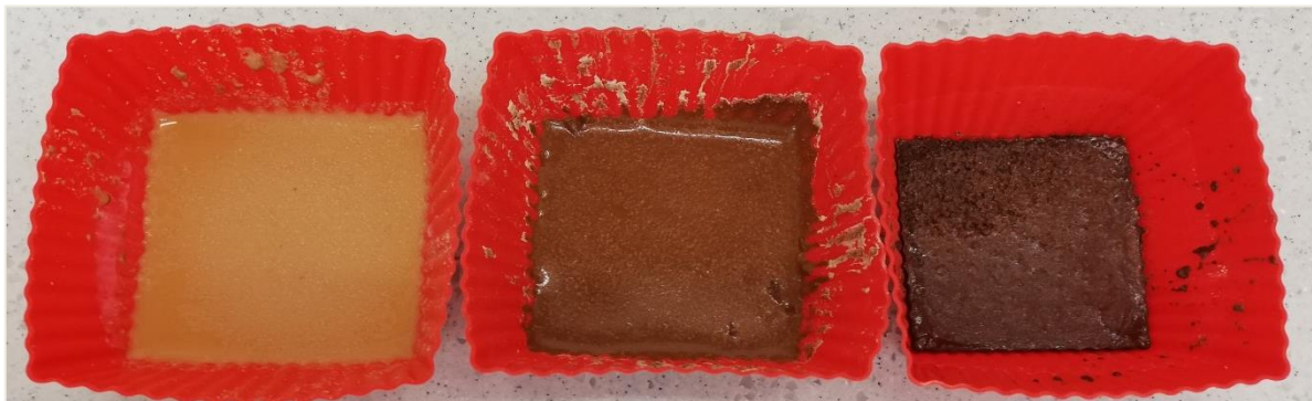
Figure 15. From left to right, aspect of the samples 1, 2 and 3 of the GP3-Granulated. For the sample 1 and 2, aspect after being synthesized. For sample 3, aspect after 20 h of synthesis.
