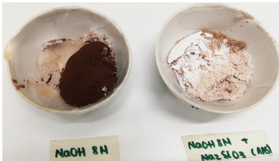
Figure 134. Aspect of the Jarosite Study 3-3 geopolymer on the 20 th curing day after crushing (physical stability test).
