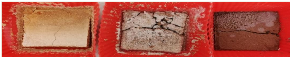
Figure 27. From left to right, aspect of the samples 1, 2 and 3 of the GP3-Granulated (29th curing day).
