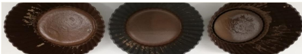
Figure 38. From left to right, aspect of the sample 1, 2 and 3 of GP6-Fine. Sample 1 and 2 after 1 h of the synthesis. Sample 3 after one day curing.
