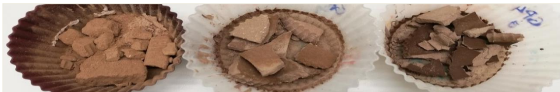
Figure 34. From left to right, aspect of the samples 1, 2, 3 of the GP4 after crushing (physical stability test; 35th curing day).
