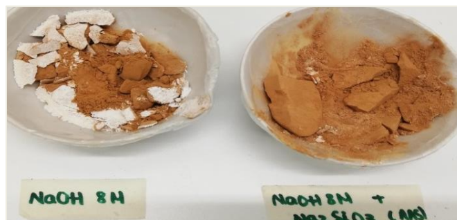
Figure 63. Aspect of the Jarosite Study 3-2 geopolymer on the 20th curing day after crushing (physical stability test).
