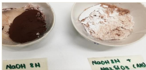
Figure 65. Aspect of the Jarosite Study 3-3 geopolymer on the 20th curing day after crushing (physical stability test).
