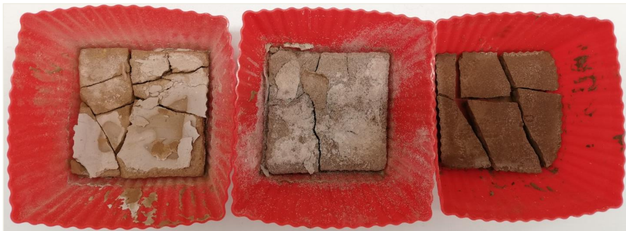
Figure 11. From left to right, aspect of the samples 1, 2 and 3 of the GP2 before crushed (42 th curing day).
